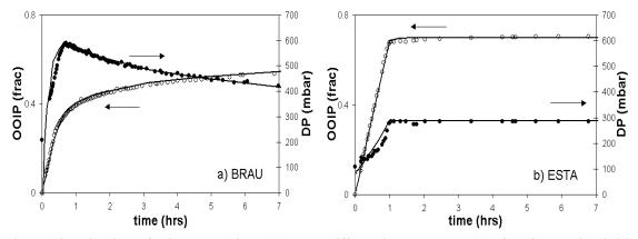
Figure 4. Kinetics of oil production ( $\circ$ ) and differential pressure ( $\bullet$ ) for forced imbibition displacements. Solid lines correspond to the history matching obtained with 1D simple porosity simulations.
