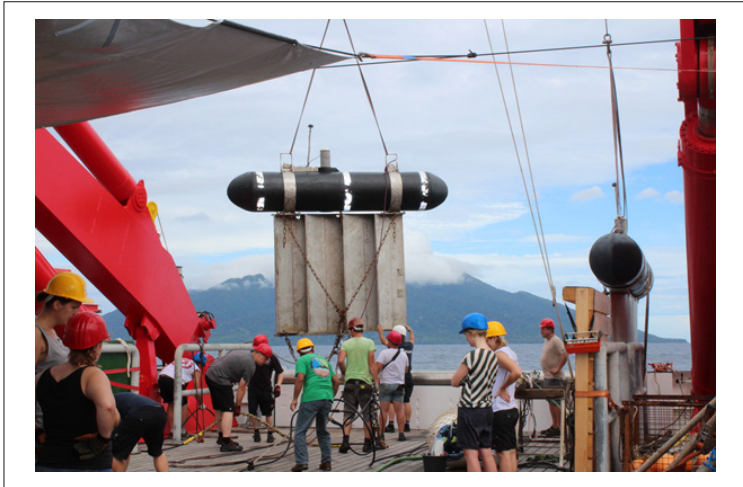
Figure 1: Deployment of the starboard paravane for the P-Cable 3D seismic system off Ritter Island during SO252. In the background there is the still intact volcano of Sakar Island (Photograph: Melanie Ray).
