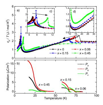
FIG. 2. a) Specific heat of the substitution series  $[(NH_4)_{1-x}K_x]_2[FeCl_5(H_2O)]$ . Inset c) resolves the low-temperature transitions and inset d) enlarges the region around the broadened high-temperature transition for x = 0.45 around 24 K. b) Temperature dependence of the polarization components  $P_a$ ,  $P_b$ , and  $P_c$  for all different potassium concentrations. The pure  $(NH_4)_2[FeCl_5(H_2O)]$  does not show a measurable polarization at  $T_S$ .
