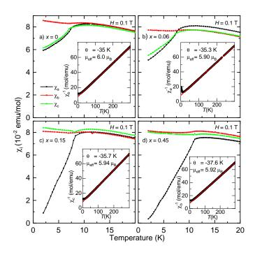
FIG. 7. Susceptibility of the substitution series  $[(NH_4)_{1-x}K_x]_2[FeCl_5(H_2O)]$  with a) x = 0, b) x = 0.06, c) x = 0.15, d) x = 0.45. The insets show the Curie-Weiss fits.
