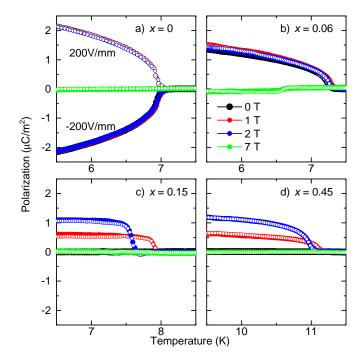
FIG. 8. Temperature dependence of the polarization  $P_a$  for the substitution series  $[(NH_4)_{1-x}K_x]_2[FeCl_5(H_2O)]$  with a) x = 0, b) x = 0.06, c) x = 0.15, d) x = 0.45. Upon cooling, electric poling fields of  $\pm 200 \,\mathrm{V \,mm^{-1}}$  (open and closed symbols, respectively) were applied and removed at base temperature. The polarization was then obtained by numerical integration of the pyrocurrent measured upon heating.
