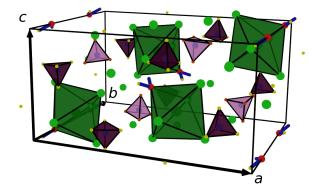
FIG. 6. Crystal structure of  $(ND_4)_2$ [FeCl<sub>5</sub>(D<sub>2</sub>O)] at 100 K (top) and 10 K (bottom). ND<sub>4</sub><sup>+</sup> tetrahedra of the same shading are symmetry equivalent.
