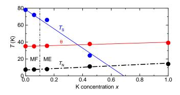
FIG. 11. Potassium concentration dependence of the transition temperatures  $T_{\rm N}$ ,  $T_{\rm S}$ , and the magnetic Curie-Weiss temperature  $\theta$  for [(NH<sub>4</sub>)<sub>1-x</sub>K<sub>x</sub>]<sub>2</sub>[FeCl<sub>5</sub>(H<sub>2</sub>O)].
