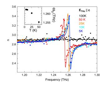
FIG. 3. Refractive index of  $(NH_4)_2$ [FeCl<sub>5</sub>(H<sub>2</sub>O)] for polarization **E** ||*c*. Below  $T_S$ , we observe the appearance of a mode at about 1.26 THz, which we attribute to a libration of the  $NH_4^+$ groups. Symbols show the experimental results, solid lines depict fits using a Lorentz oscillator. The inset resolves the temperature dependence of the eigenfrequency of this mode.
