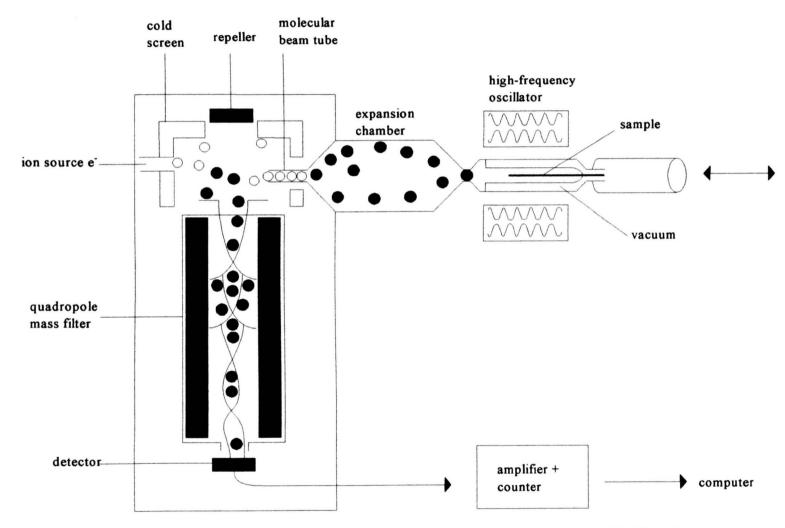
Figure 1.2 Schematic diagram of the Horizon 400X pyrolysis mass spectrometer (Modified from Magee, 1993)
