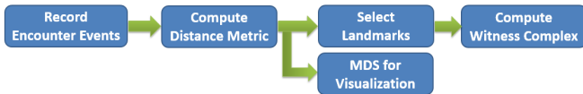
Fig. 5. Block diagram of the topological estimation of an environment based on encounter events and witness complex
