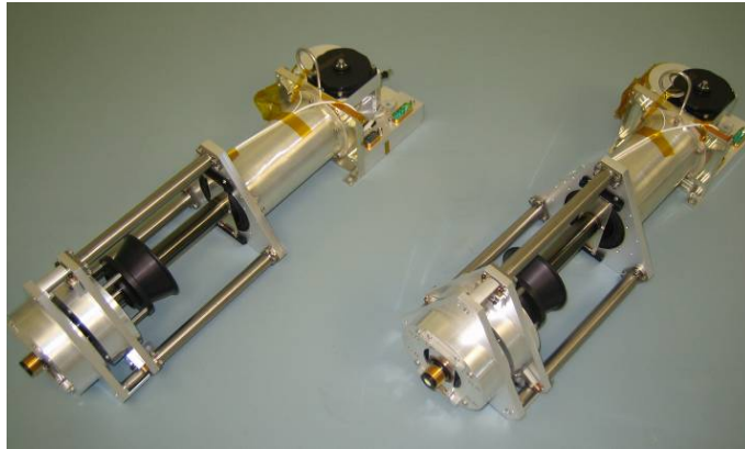
Stacer booms to be used for deployment
