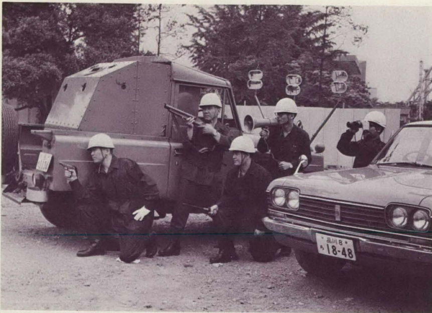
Crime Combat Team officers use special armored vehicle as cover. This vehicle, equipped with ports for firing gas guns or other weapons from the rear and sides, has multiple rearview mirrors since it is employed by backing slowly toward a dangerous subject.
