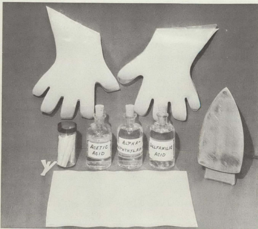
Chemicals and materials necessary for conducting a gunpowder residue test.
