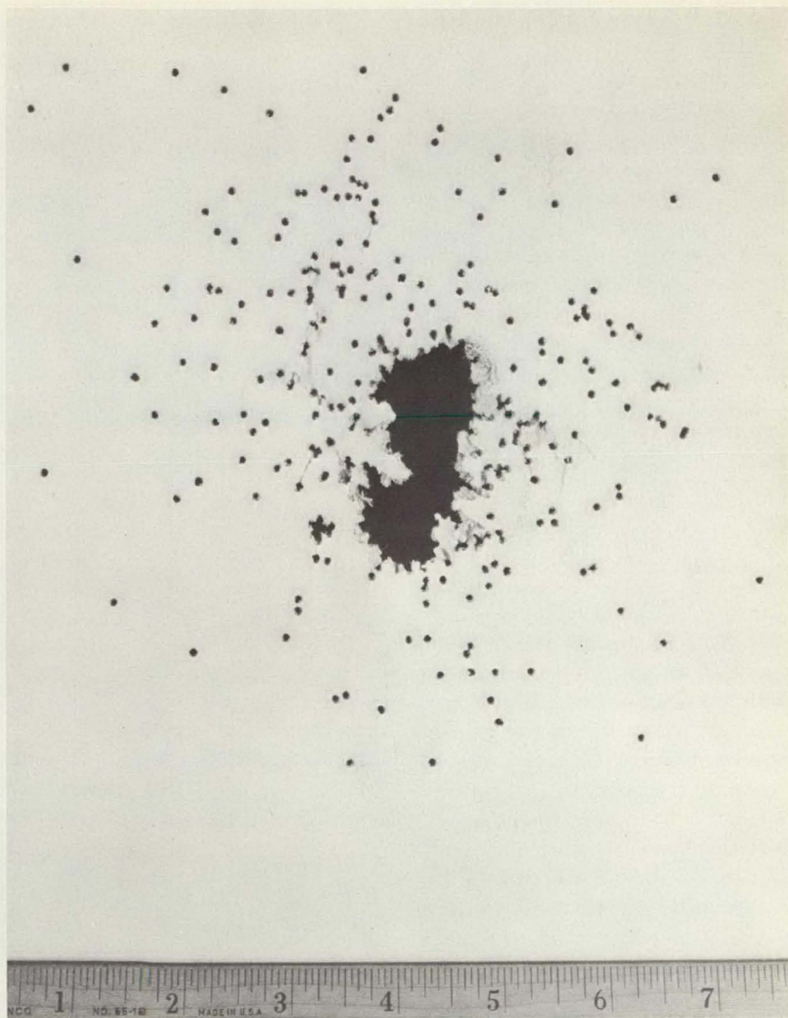
Test pattern from 7 yards. Note pattern approximately 7 inches in diameter.
