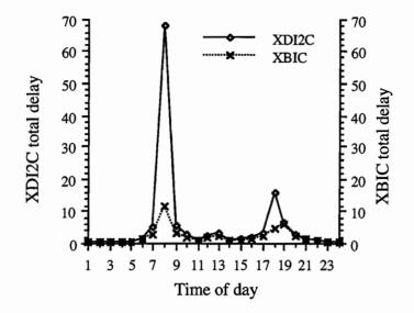
Figure 4.16. X intersection, hourly total delay comparison between BIC and DI2C
