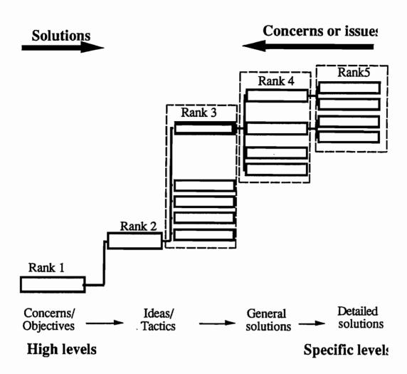
Fig C4. The basic concept of the Hierarchy of Objective Techniques (HOT) diagram (Ref 15).
