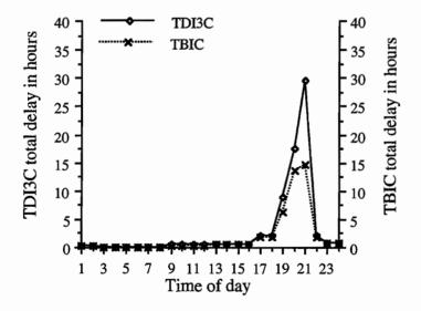
Figure 4.21. T intersection, hourly total delay comparison between BIC and DI3C
