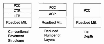
Figure 6.1. Design of reduced number of layers and full-depth sections to expedite pavement construction (Ref 1)
