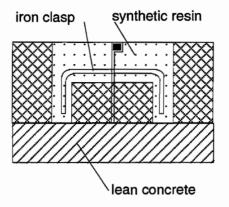
Figure 6.3. Longitudinal joint construction in prefabricated portland cement concrete slab
