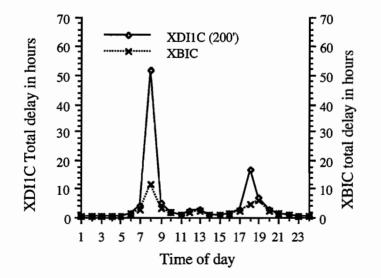
Figure 4.15. X intersection, hourly total delay comparison between BIC and DI1C
