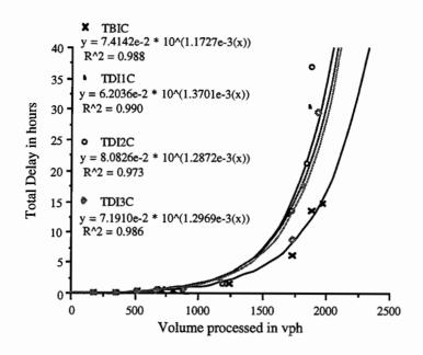
Figure 4.22. T intersection, total delay vs volume processed
