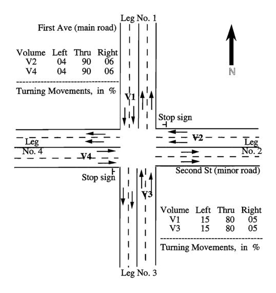
Figure 4.9. X intersection before improvement configuration
