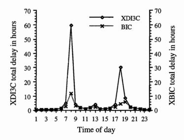
Figure 4.17. X intersection, hourly total delay comparison between BIC and DI3C
