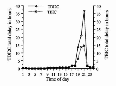
Figure 4.20. T intersection, hourly total delay comparison between BIC and DI2C
