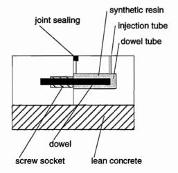
Figure 6.2. Transverse joint construction in prefabricated portland cement concrete slab
