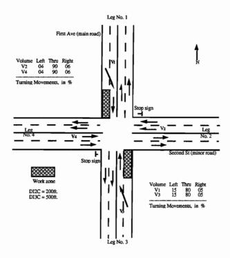
Figure 4.12. X intersection during improvement 3 configuration
