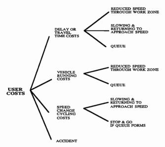
Figure 4.3. Additional user-cost components resulting from work zone interruption
