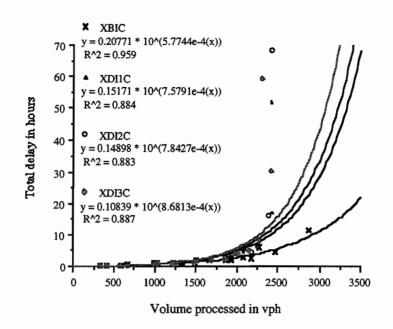
Figure 4.18. X intersection, total delay vs volume processed
