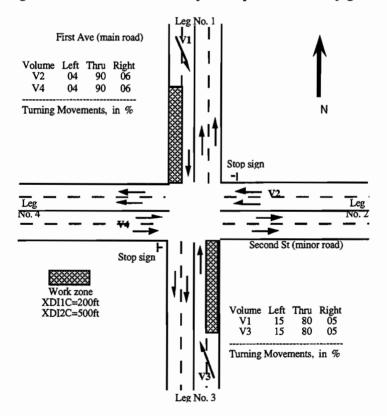
Figure 4.11. X intersection during improvement 1 and 2 configuration
