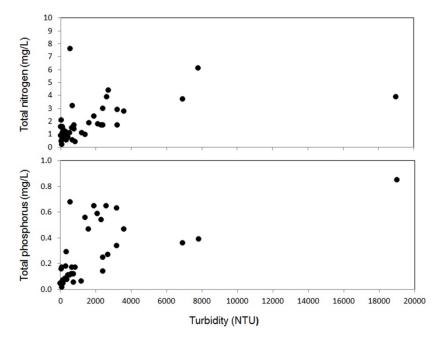
Figure 10. Turbidity (within the range 0 to 20000 NTU) versus total nitrogen and phosphorus
