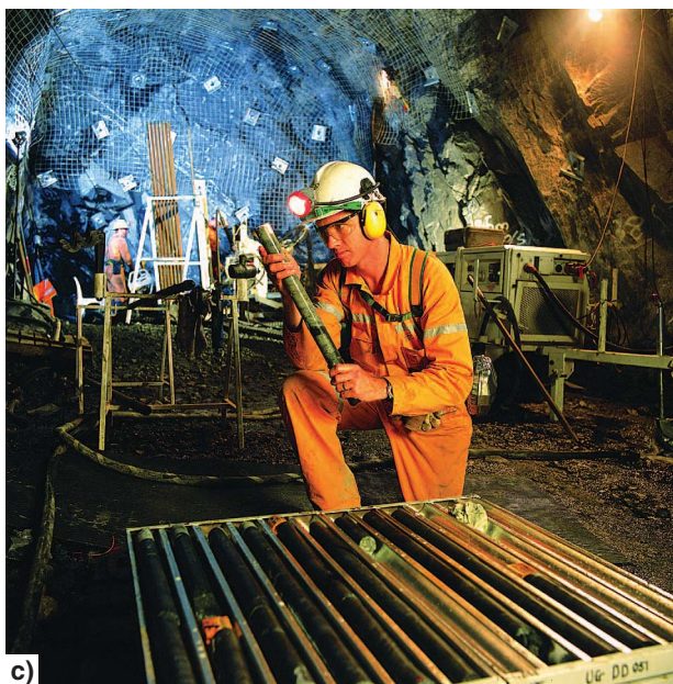
Figure 14. Mining operations at Greenbushes: a) the giant Cornwall tantalum-tin openpit that is over 200 m deep; b) construction of the Cornwall pit decline; c) examining diamond drillcore at the Cornwall pit decline; d) mining operations in the Cornwall openpit (photos (a)–(c) courtesy Sons of Gwalia Ltd)
