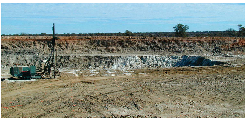
Figure 22. Blast hole drilling at the Bald Hill openpit (looking west)
