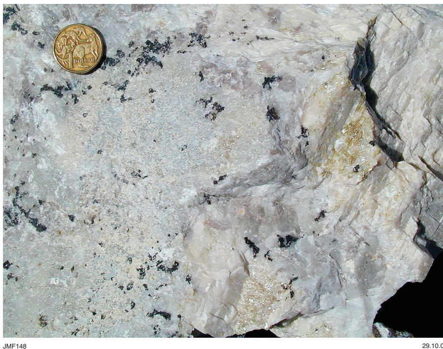
Figure 72. Bald Hill pegmatitic tantalum ore comprising massive albite, quartz, and microcline, with lesser amounts of mica and spodumene. The visible black material is mainly manganese staining
