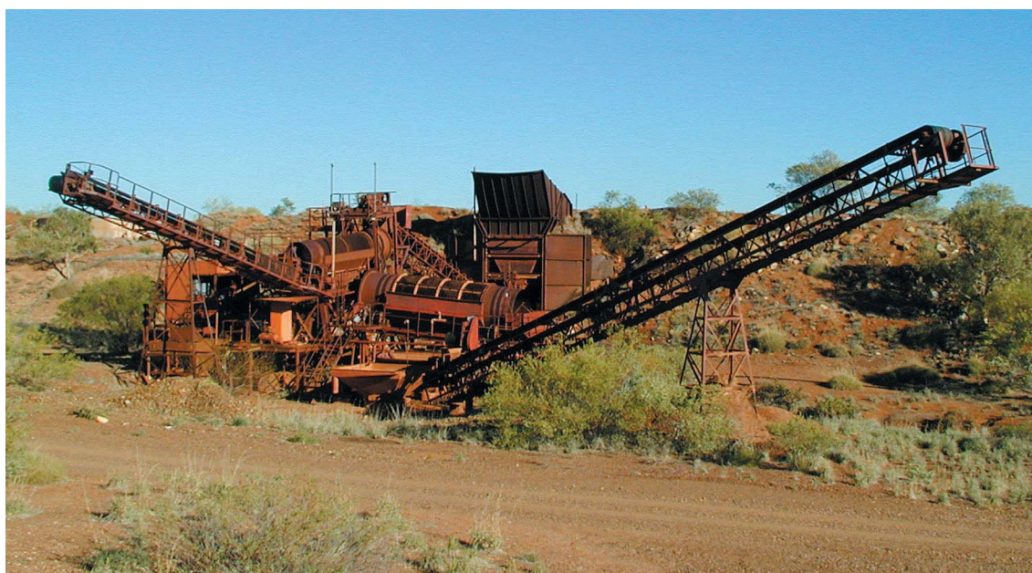
Figure 32. Disused alluvial tin–tantalum processing plant at the Pilgangoora Alluvials deposit
