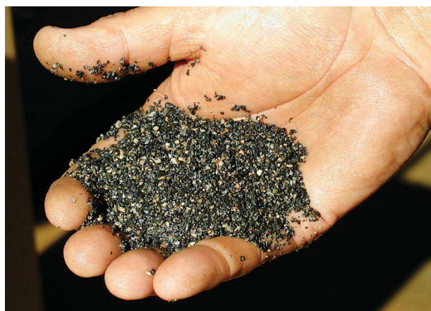
Figure 29. Coarse jig concentrate of tantalite and microlite (25–80% Ta 2 O 5 ) at the Dalgaranga plant
