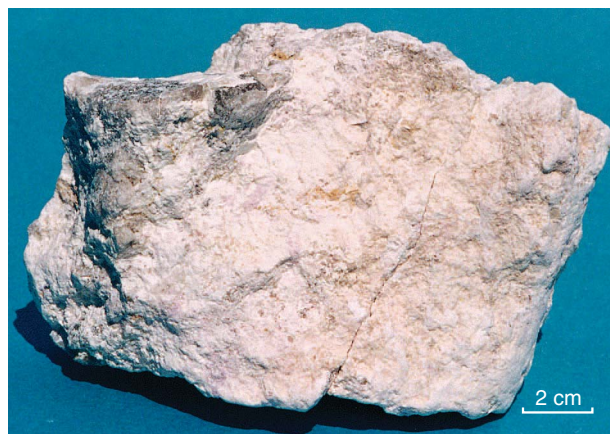
Figure 8. Highly kaolinized tantalum ore at Wodgina that has been derived from deep weathering of feldspar in pegmatites in the Mount Tinstone orebody
