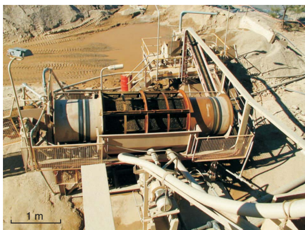
Figure 26. Trommel screening the ore feed to the Dalgaranga plant; the minus 9 mm feed is sent to the ball mill for grinding, oversized ore is retained for retreatment, and fines are removed to the tailings dam
