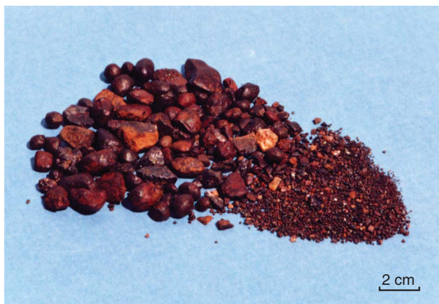
Figure 31. Wodgina alluvial tin–tantalum concentrate (11.1% Sn, 5.8% Ta)
