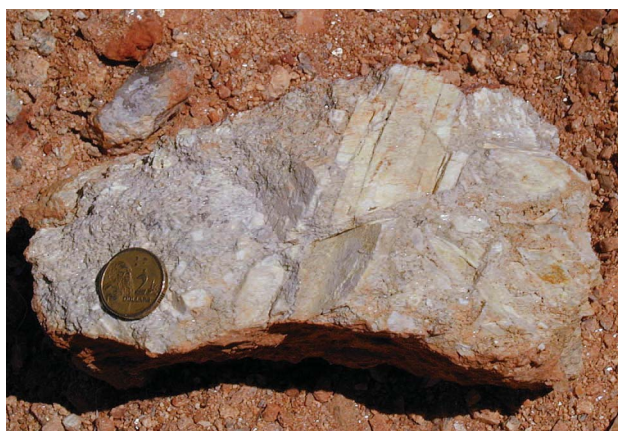
Figure 89. Replacement of cleavelandite (right) by sugary albite (left) at the Tantalus prospect
