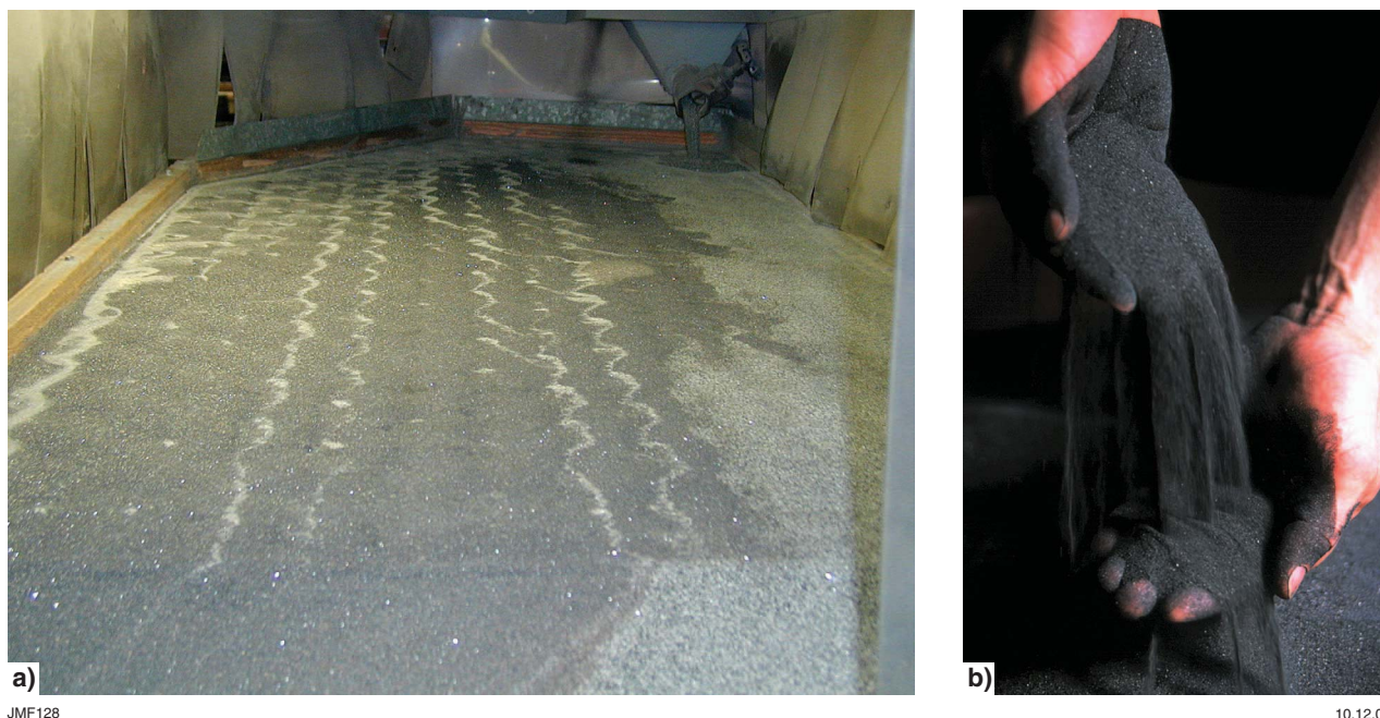
Figure 17. Secondary processing of the Greenbushes tantalum-tin concentrate: a) dry gravity separation on an air shaking table; b) final high-grade tantalum concentrate at 30% Ta 2 O 5 (photo (b) courtesy Sons of Gwalia Ltd)
