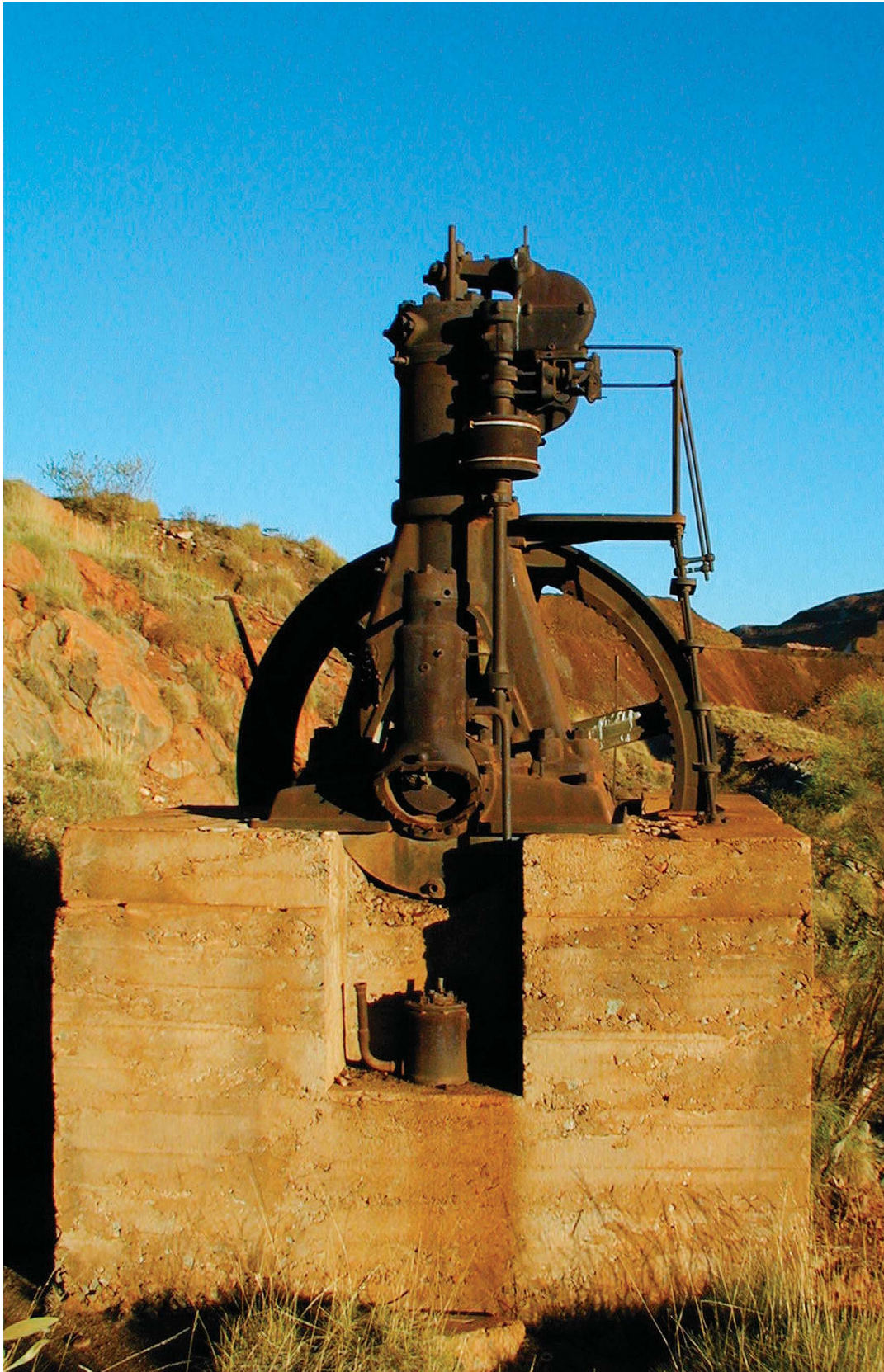
FRONTISPIECE: Historic pump at the Wodgina tantalum-tin mine. Brought from Port Hedland by camel train about 1905, this vintage steam pump was used for many years pumping water and providing motive power for ore crushing
