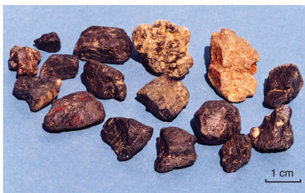
Figure 27. Pebble-sized tantalite (dark) and microlite (light) concentrate that has been trapped by the trommel screen at the Dalgaranga plant
