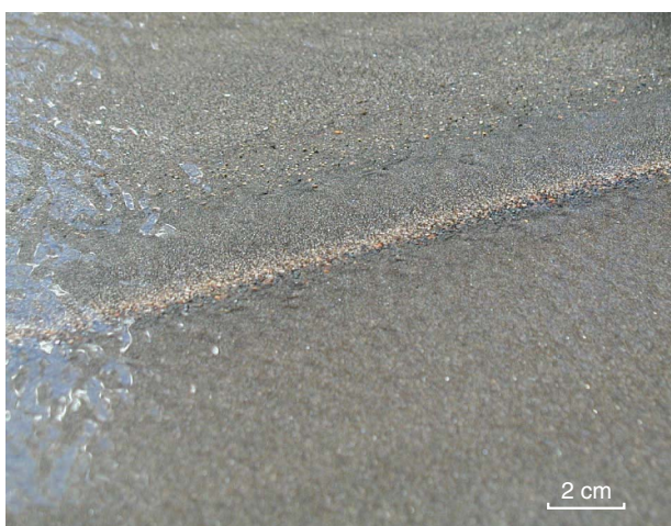
Figure 28. Tantalite and microlite streams on a wet shaking table at the Dalgaranga plant
