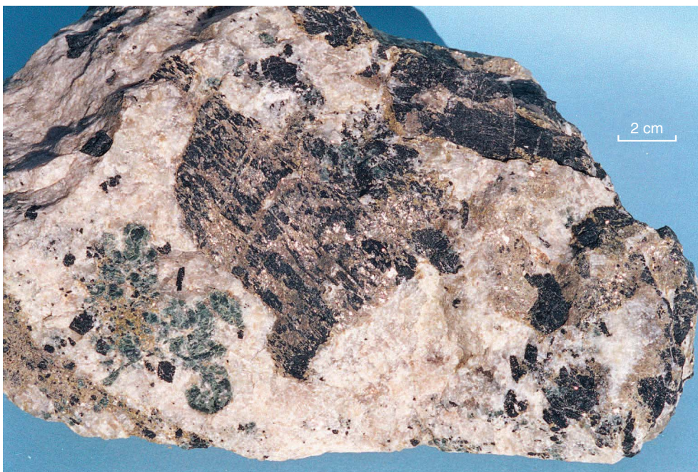
Figure 95. High-grade tantalum ore from Pegmatite C, Cornwall openpit. Visible minerals: albite (white), quartz (pale grey), tourmaline (black), muscovite (yellow with reflective plates), and apatite (grey-green)
