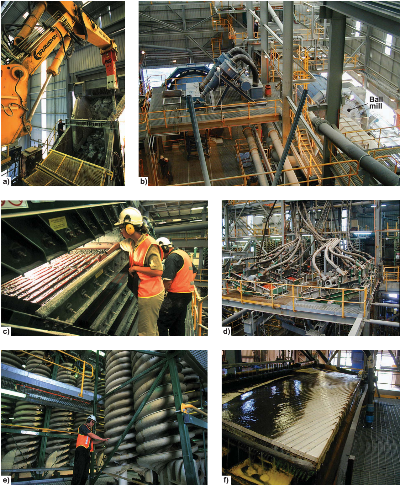
Figure 16. Primary processing of the Greenbushes tantalum–tin concentrate: a) primary ore crusher; b) ball milling minus 12 mm crushed ore to sand-sized particles (0.5 – 1.0 mm); c) checking the classification screens; d) banks of Derrick screens separating coarse, unliberated tantalum ore particles for regrinding; e) banks of spiral concentrators effecting fine gravity separation of the tantalum ore; f) wet shaking tables for primary ore upgrading to 4–6% Ta 2 O 5 concentrate (photos (a), (c), and (e) courtesy Sons of Gwalia Ltd)
