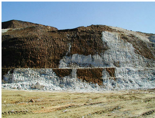
Figure 63. Deeply weathered, kaolinized pegmatite and host psammitic metasedimentary rocks at the Mount Cassiterite openpit (looking west)
