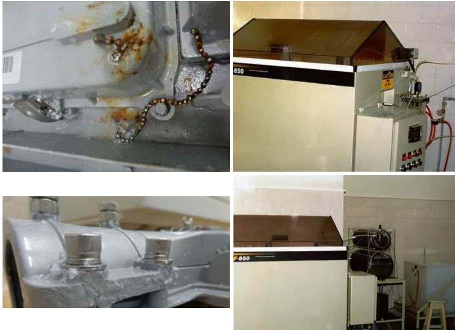
Fig. 3. LAL salt fog test equipment and results (photos from author)
