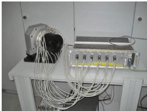
Fig. 1. Tuneable colour light source for calibration purpose: on the left is the sphere with LEDs around the output port; on the right is the 24 channel DC source of power
