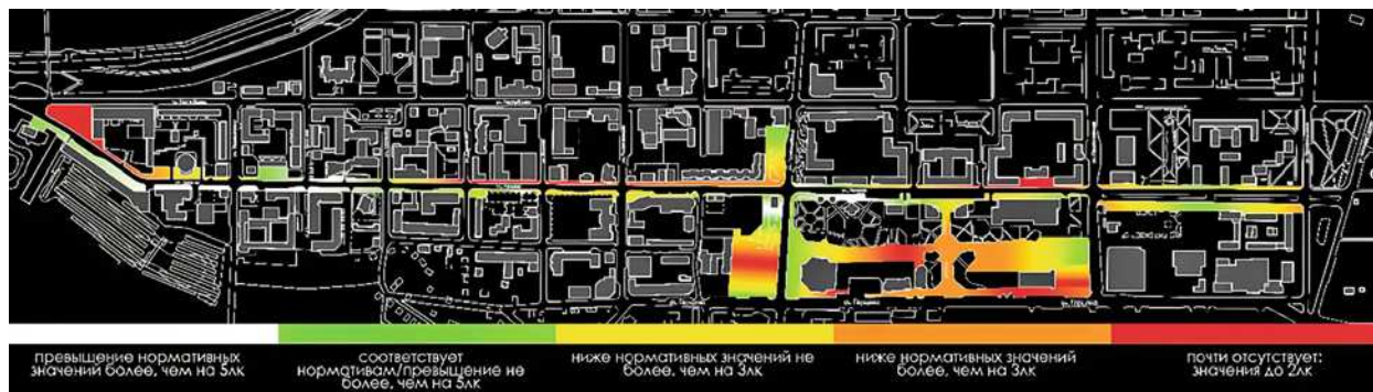
Fig. 1. Scheme of compliance of the illuminance level of the Lenin st. with norms of SP 52.13330.2016 based on the report of instrumental observation of priority objects of urban environment (August 2017)
