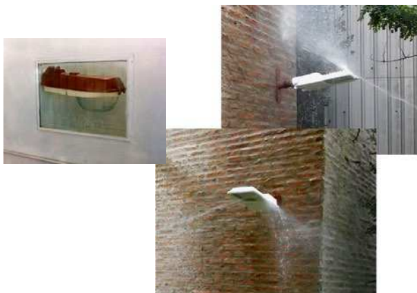
Fig. 4. IP test: air (left) and water tightness (right) (photos from author)
