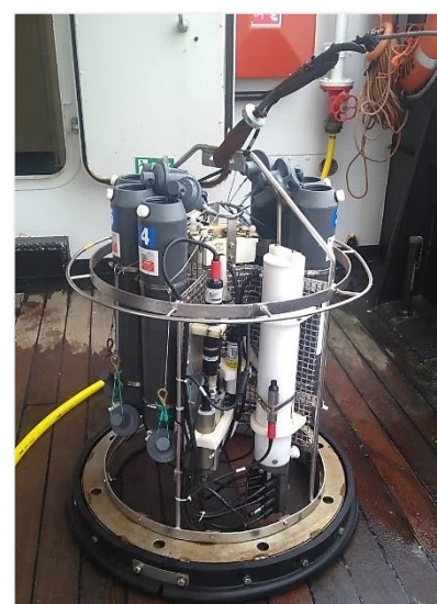
Figure 6: Niskin bottles and CTD mounted on a carousel on board of RV Simon Stevin.
