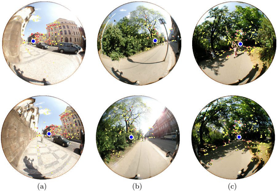
Fig. 3. Examples of pairs of images (two consecutive frames) from top to bottom in the CITY WALK sequence. Blue circles represent the epipoles and yellow dots are the matches supporting this epipolar geometry. Red dots are the matches feasibly reconstructed as 3D points. (a) contains multiple moving objects and large camera rotation. (b) contains large camera rotation and tentative matches on bushes. (c) contains tentative matches mostly constructed on a complex natural scene.
