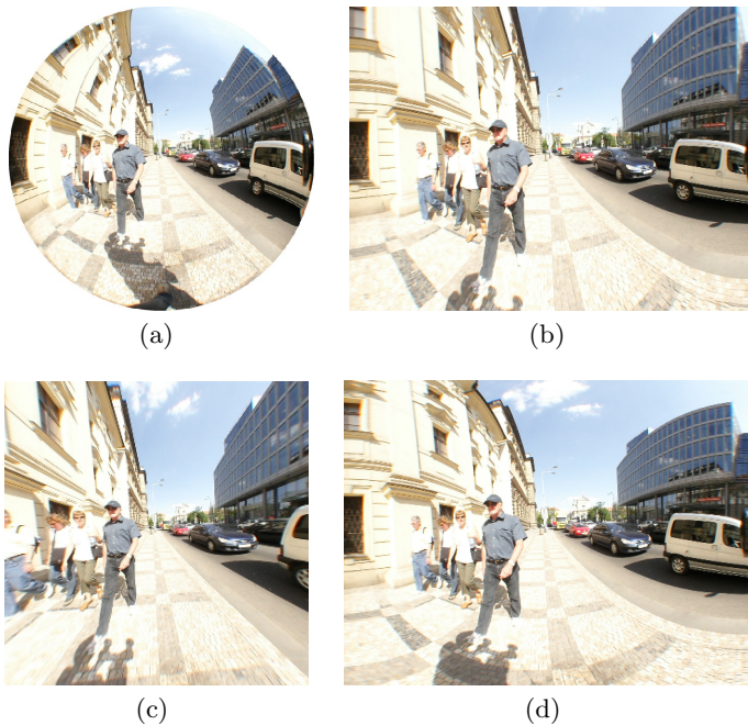
Fig. 5. (a) Original omnidirectional image (equiangular). (b) Central cylindrical projection. (c) Perspective projection. (d) Non-central cylindrical projection. Note there is a large deformation at the borders of the perspective image and at the top and bottom borders of the central cylindrical image. The borders of the non-central cylindrical image are less deformed.
