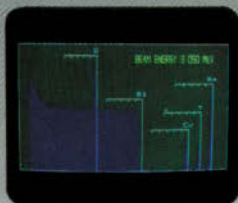
Variable beam energy for oxygen depth profiling.
