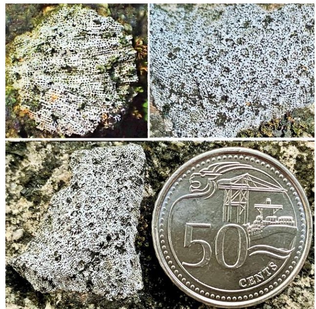
Fig. 12. Hard coral fragments found exposed within mortar. (Photographs by: Lau Wing Lup).
