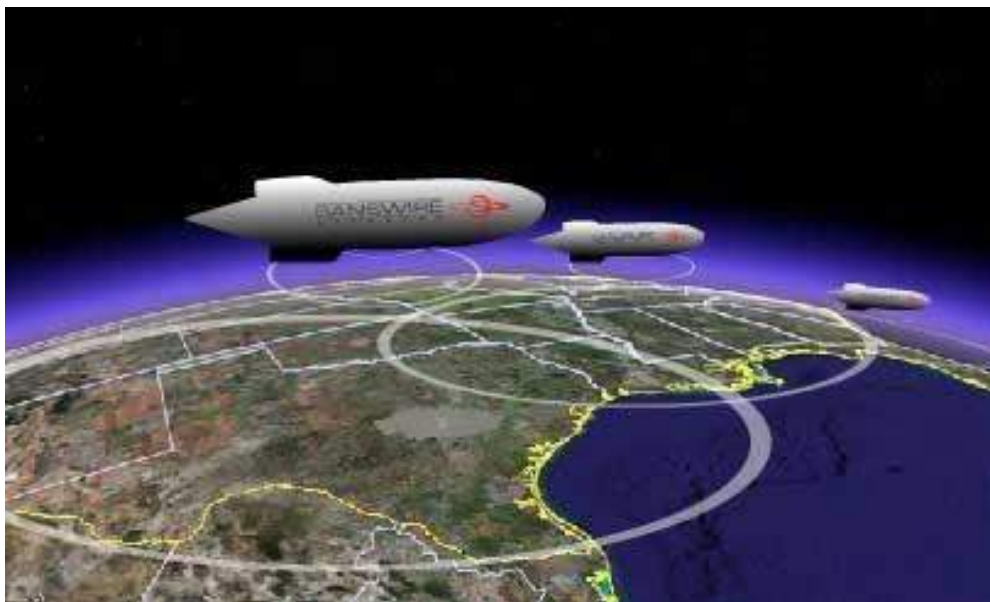
Example of coverage provided by a constellation of three Sanswire Stratellite airships along the US Gulf Coast. Source: Sanswire
