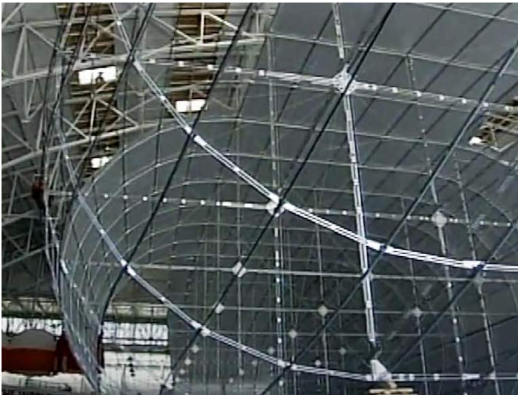
The rigid aluminum frame of the Sanswire One prototype during assembly, with some hull panels in place. Source: Sanswire.
