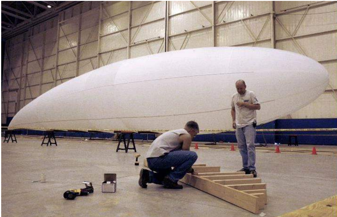
Sanswire 2A Technology Demonstrator inflated, but without the fin/rudder system installed. Source: AP via Tahoe Daily Tribune
