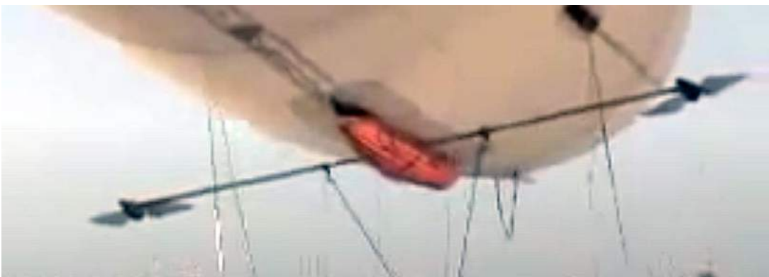
Equipment pod and two propulsion propellers. Source: Screenshot from Sanswire Dec 2006 YouTube video
