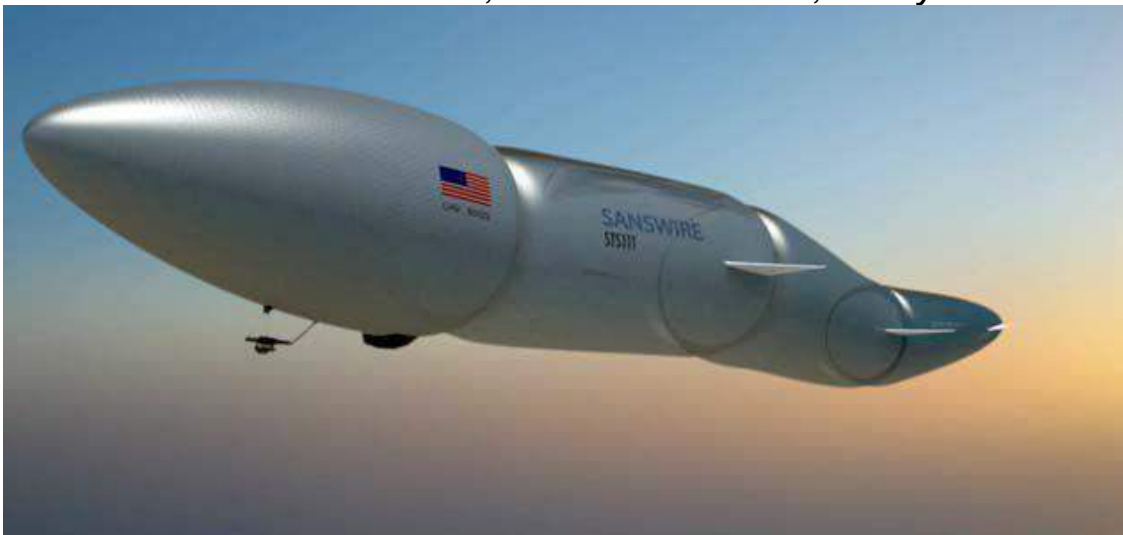
Artist's rendering of the STS-111, with carbon fiber winglets on all of the trailing segments to aid with lift, steering and overall stability.
