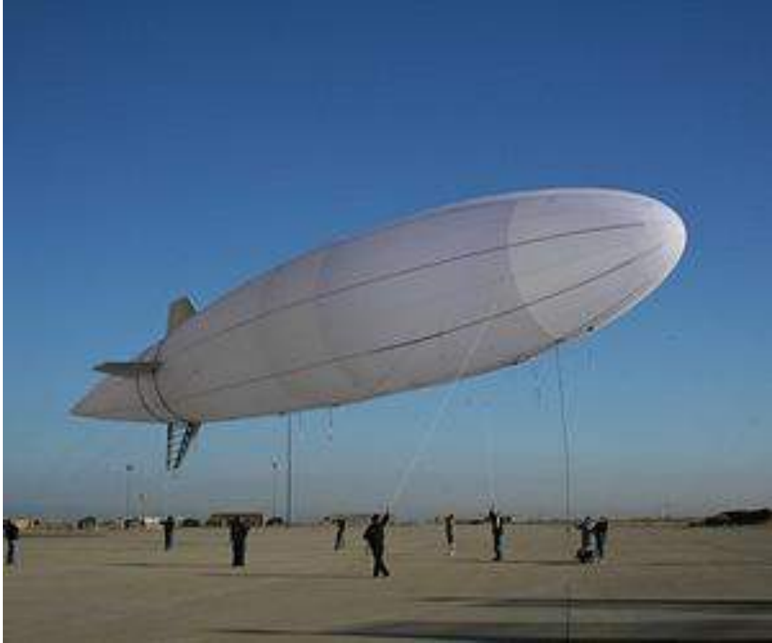
Sanswire 2A Technology Demonstrator tethered test. Source: The Register
