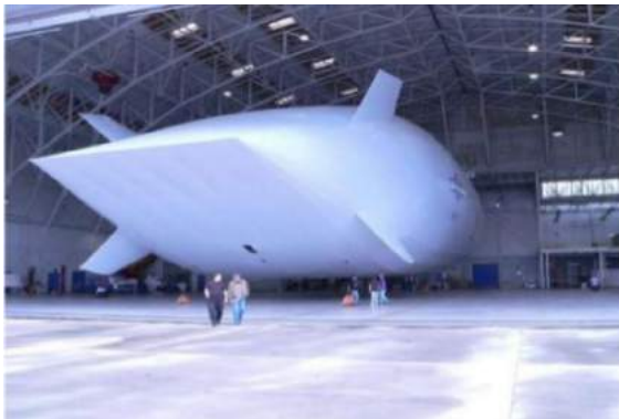
In-hangar float test of the Sanswire One prototype. Source: Sanswire
