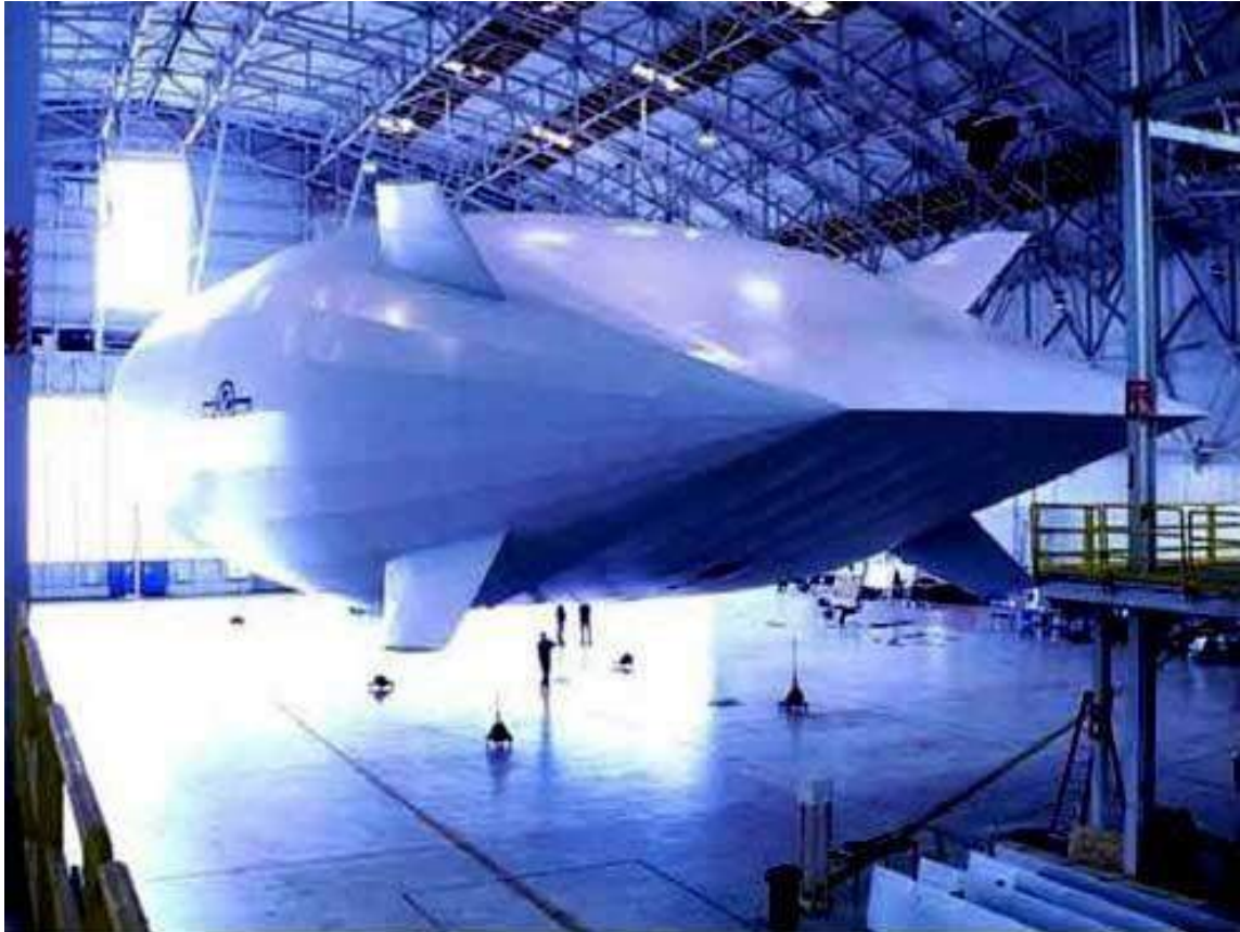
In-hangar float test of the Sanswire One prototype. Source: Sanswire
