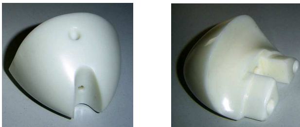
Fig. 8 The part model created by means of Rapid Prototyping
