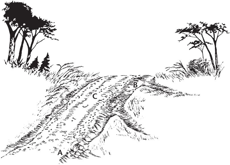
Figure 7. Water Turnout Construction.
