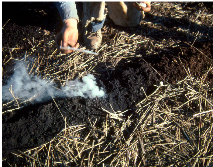
Figure 10-13.—Soils high in manganese can be confirmed as nonorganic with the application of cold, 3 percent hydrogen peroxide, which will evolve a whitish cloud of gas in the presence of manganese oxide.
