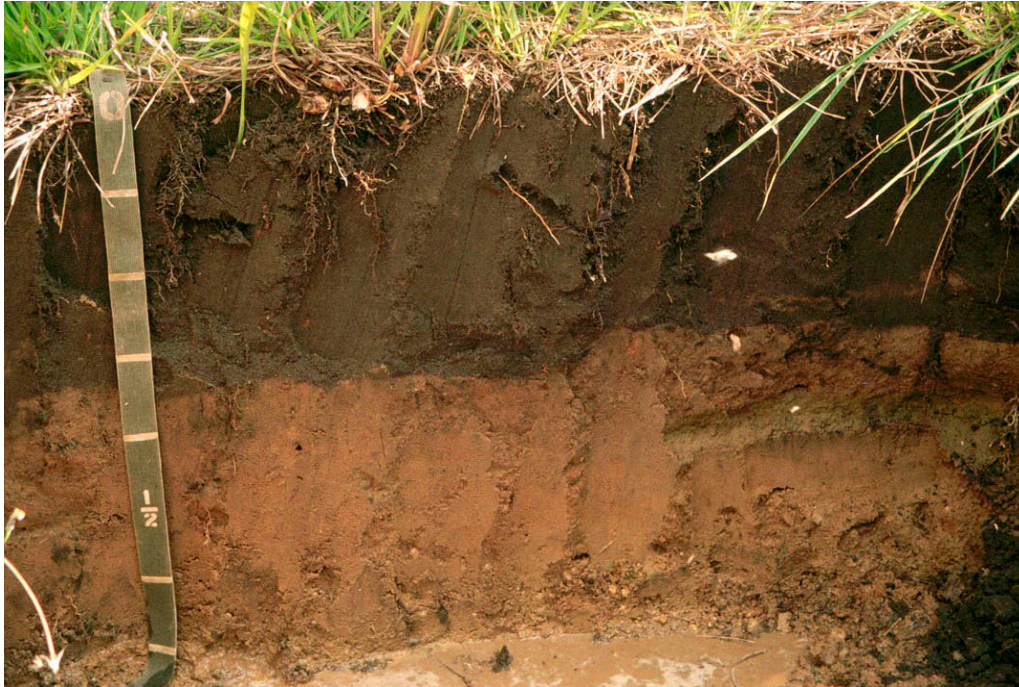
Figure 10-4. —An anomalous, bright, sandy hydric soil within 200 ft (8 m) of a tidal marsh. The surface layer is thick because it has been plowed. From 0 to 13 in (0 to 32 cm), it is 10YR 3/2 with few fine distinct 7.5YR 3/4 redox concentrations occurring as soft masses. The soil has a 10YR 4/6 matrix at a depth of 13 to 24 in (32 to 70 cm).
