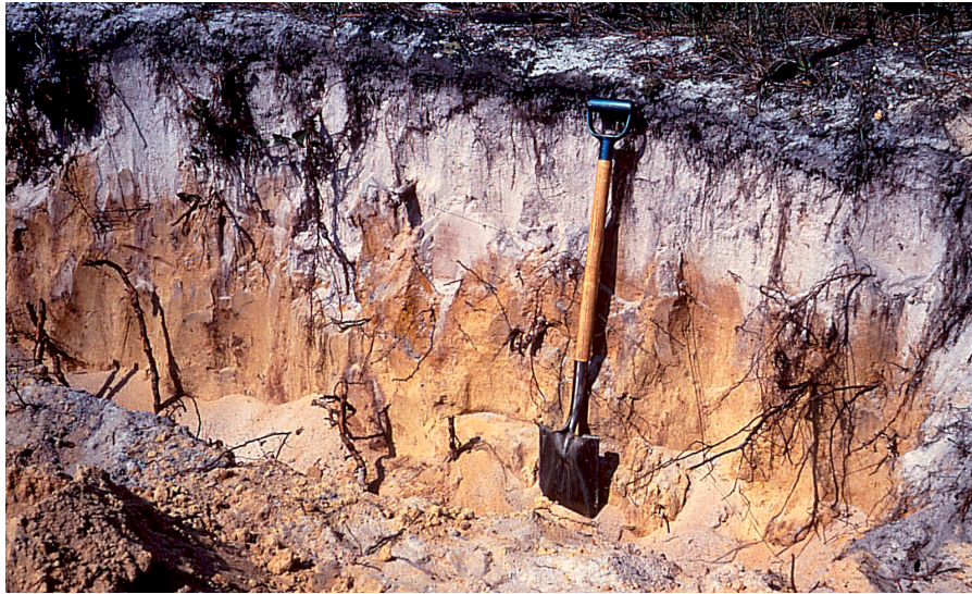
Figure 10-9.—A dry, coastal plain, sandy soil with a thick, gray E horizon. This soil may be mistaken for a hydric soil because it has a thick, gray E horizon.
