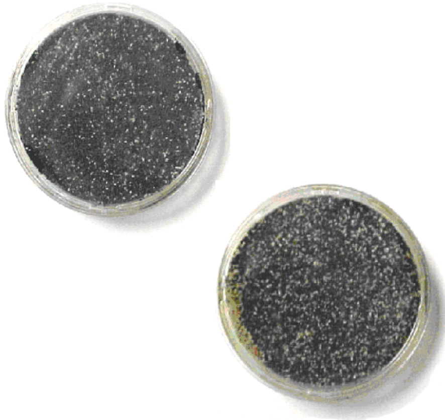
Figure 6-3.—On the left, 70 percent of sand grains coated or masked by organic compounds; on the right, 50 percent of sand grains coated or masked by organic compounds.
