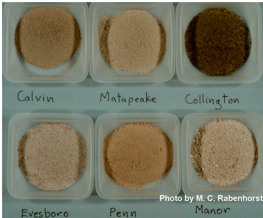
Figure 3-1. —Note the variety in color of uncoated mineral grains, which contribute to the color of soils. Iron oxides were removed from these soil materials, which are from six different soil series that formed in a variety of parent material.
