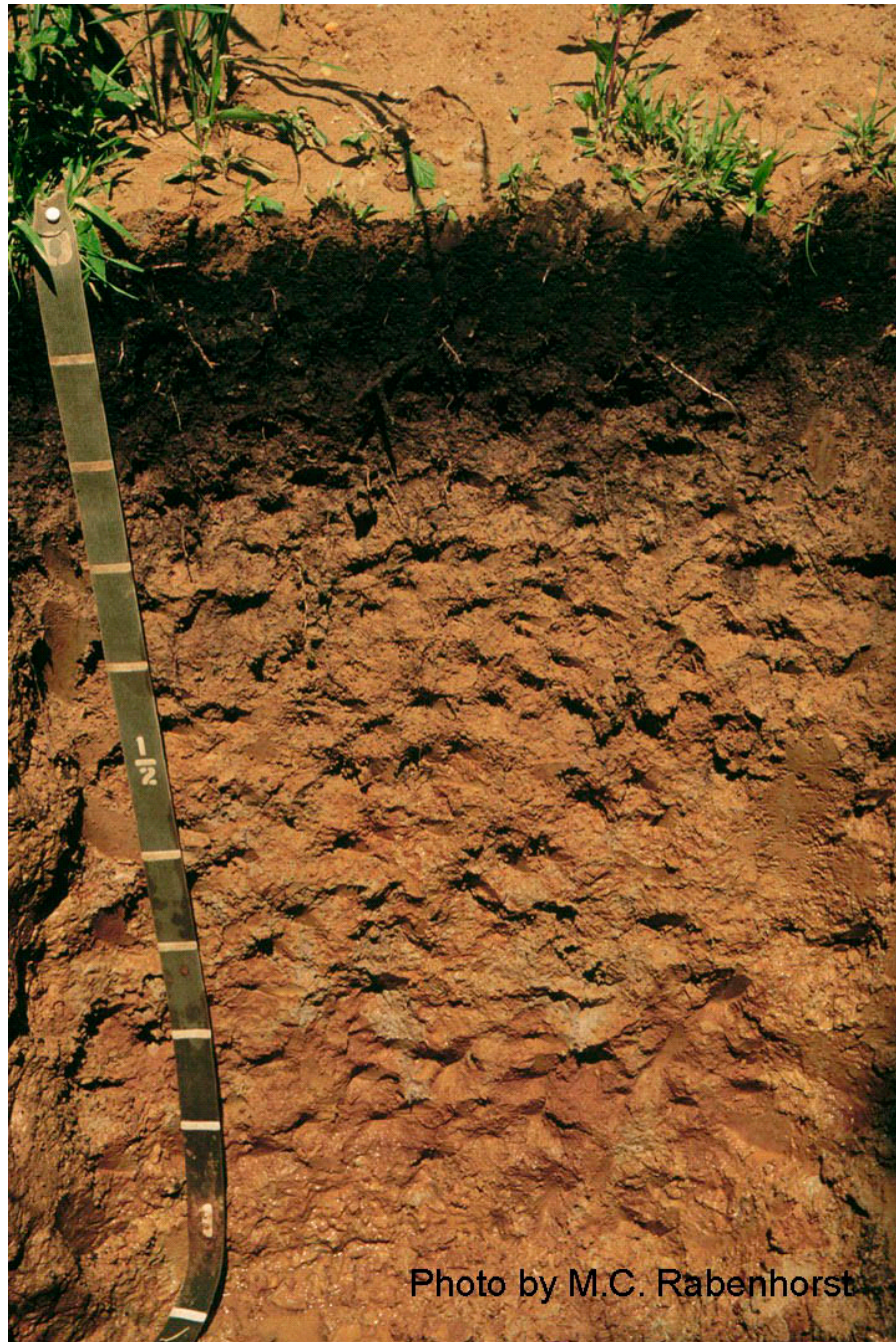
Figure 10-3.—An anomalous, bright, loamy hydric soil from a University of Maryland study site. The typical matrix is 10YR 5/3 or 4/4 at a depth of 8 to 20 in (20 to 50 cm) and 10YR 4/6 at a depth of 20 to 32 in (50 to 80 cm). It has common medium distinct 10YR 5/2 redox depletions and common medium distinct 7.5YR 4/6 redox concentrations, which occur as soft masses.
