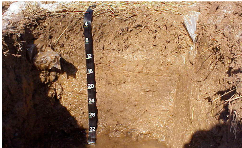
Figure 10-2. —A hydric soil formed in alluvium derived from red parent material. This soil is on a flood plain at a Mid-Atlantic Hydric Soils Committee study site. The red parent material was confirmed by CCPI testing. The profile is sufficiently wet for a very long period of time and meets Field Indicator F3 (Depleted Matrix).
