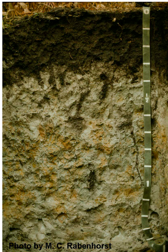
Figure 3-10.—Soil profile from which iron has been largely removed, resulting in a gray Btg horizon.
