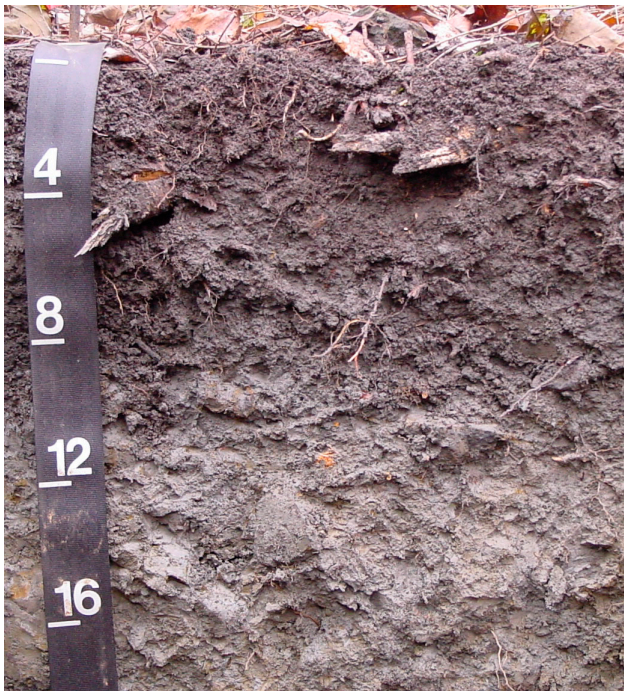
Figure 10-15.—A closeup of burnt shale showing the reddish parachanners and pseudomorphs that can be misinterpreted as redox concentrations.
