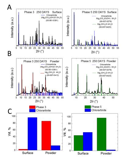
**Figure 7.** Phase composition of the surface and bulk (powder) of Phases 3 and 5 at 250 days of sample ageing.
