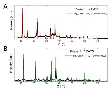
Figure 3. XRD patterns for magnesium oxychloride cement (MOC) Phases 3 and 5 after 7 days.
