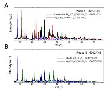
Figure 4. XRD patterns of MOC Phases 3 and 5 after 50 days.
