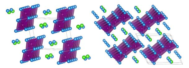
**Figure 1.** Crystal structures of Phase 3 (left) and Phase 5 (right). Mg atoms are located in the centers of distorted octahedra formed by oxygen atoms. Cl atoms—green; O atoms—blue. Green-blue spheres in the Phase 5 structures correspond to a mixed site occupied by chloride anions and water molecules (hydrogen atoms are not shown).
