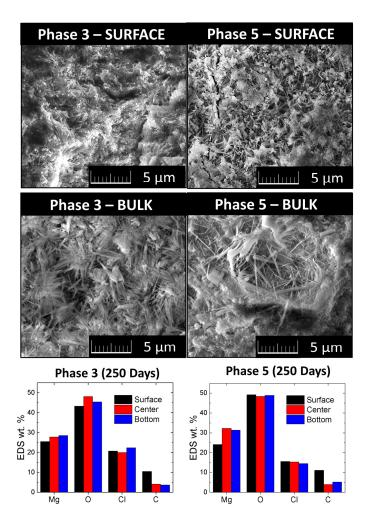
**Figure 8.** SEM micrographs of the surface and bulk (fracture surface) of samples of Phases 3 and 5 scanned after 250 days of ageing. The EDS measurements were performed from the surface, center, and bottom of the samples.
