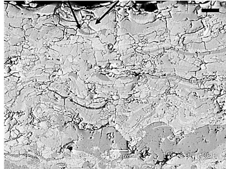
Figure 12. SEM image of microstructural details of the end electrode layer of the five-layered cell. Within the LSM layer, light grey areas predominate which are rich in La and Sr, while dark grey areas appear rich in Mn. The scale bar attached on the upper right corner of the Figure corresponds to 10 \mu\text{m} .
