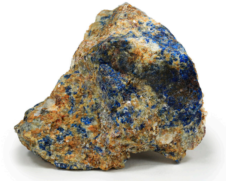
Figure 1. Bright blue CO 2 -rich, SO 4 -bearing lazurite with orange diopside in metasomatic rock. Sample 6. Field width: 9 cm. Photographer: Anastasia D. Kasatkina.
