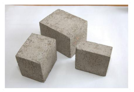
**Figure 11.** Concretes from magnesium-containing rocks of the Yoko–Dovyren massif. Large one have size  $20 \times 12 \times 10$  sm<sup>3</sup>.
