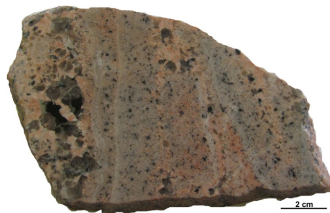
Figure 3. Striped (layered) texture of Li-F-granites (polished hand specimen). (Lypikko).
