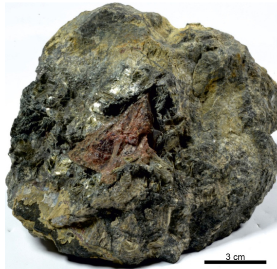
Figure 13. Brownish-red helvite— (\text{Mn}_4(\text{Be}_3\text{Si}_3\text{O}_{12})\text{S}) crystal in aposkarn greisen with magnetite. Lupikko. [52].
