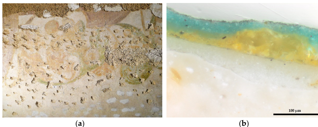
Figure 2. (a) Photo of the area where samples G4 and G5 were collected; (b) cross-section of sample G4 with a bluish-green copper pigment layer on top of the sample, magnification \times 200 .
