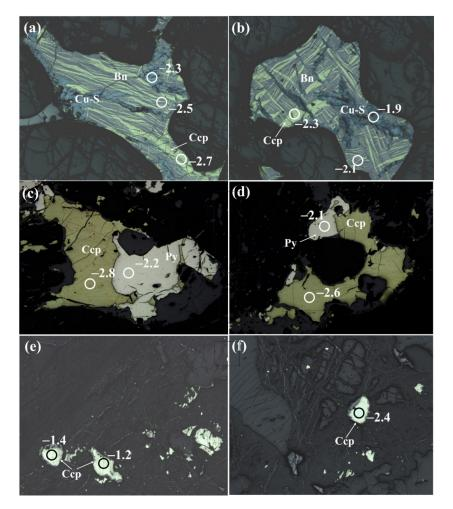
**Figure 13.** Sulfur isotopic composition of sulfides from Ozernoe (**a**–**d**) and Baronsky (**e**,**f**) deposits. Sites of analysis are shown by circles with a diameter 100  $\mu$ m, numbers show  $\delta^{34}$ S values in ‰. Minerals: Py—pyrite, Ccp—chalcopyrite, Bn—bornite, Cu-S—copper sulfide replacing bornite.
