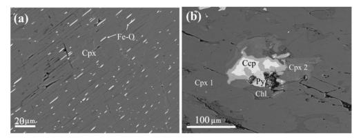
**Figure 4.** Clinopyroxene in samples of clinopyroxenites III (**a**) and I (**b**). (**a**) Thin plates of Fe-O phase in primary clinopyroxene (Cpx); (**b**) secondary clinopyroxene (Cpx 2) in intergrowths with chlorite (Chl), pyrite (Py), and chalcopyrite (Ccp) in primary clinopyroxene (Cpx 1).
