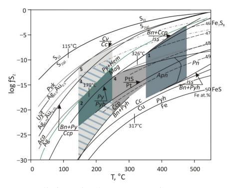
**Figure 15.** Sulfur fugacity dependence on temperature for Fe-S-O, Cu-Fe-S, Au–Ag–S, and Pt-S systems, and  $\log fS_2$  and T estimations for different associations at Ozernoe occurrence. Minerals: Bn—bornite, Ccp—chalcopyrite, iss—bornite-chalcopyrite solid solution, Py—pyrite, Pyh—pyrrhotite, Mag—magnetite, Hem—hematite, Pn—pentlandite, Apn—argentopentlandite, Pvk—petrovskaite; Uyt—uytenbogaardtite; Aca—acanthite; Cc—chalcocite; Cv—covellite.
