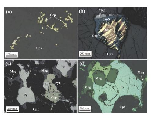
**Figure 2.** Relationships of main ore minerals in the samples of clinopyroxenites I (**a**), II (**b**), and III (**c**,**d**). Bn—bornite, Ccp—chalcopyrite, Cpx—clinopyroxene, Cu-S—secondary copper sulfide, Mag—magnetite, Py—pyrite, Pyh—pyrrhotite.
