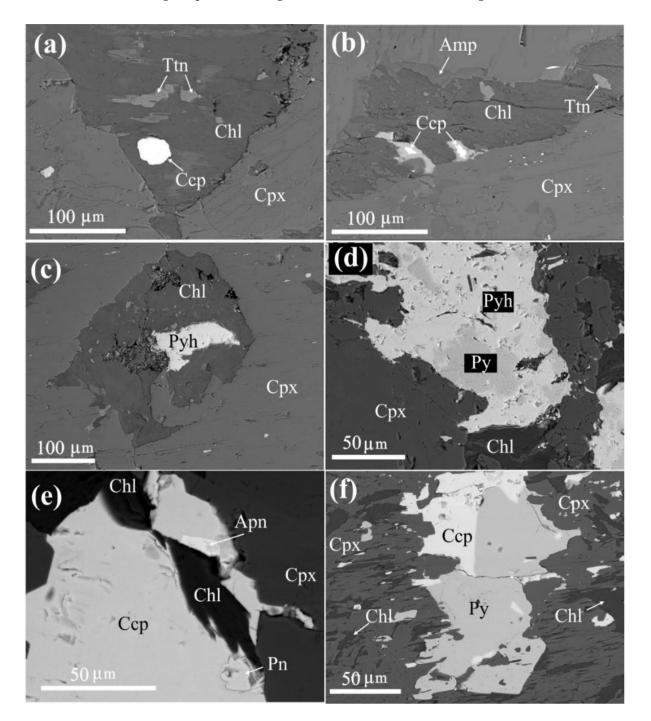
chalcopyrite (Figure 2c). Chalcopyrite was found to contain inclusions of pentlandite and argentopentlandite  $Ag(Fe,Ni)_8S_8$  of 10–15  $\mu$ m in size (Figure 9e, Table 9, No 16, 17).
