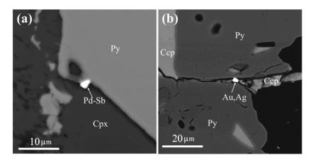
**Figure 12.** Noble metal minerals in clinopyroxenite III. (**a**) Crystals of palladium antimonide (Pd-Sb) on the surface of pyrite grain (Py); (**b**) Ag-Au particle (Au,Ag) (Table 10, No 14) in chalcopyrite (Ccp) at the contact of two pyrite (Py) grains.
