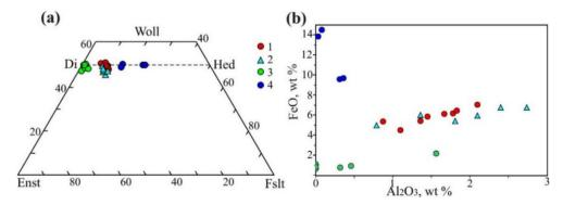
**Figure 3.** Diagrams of composition of clinopyroxenes (**a**) and contents of FeO-Al<sub>2</sub>O<sub>3</sub> (**b**) in primary and secondary clinopyroxenites. Primary clinopyroxene from clinopyroxenites I (1), II (2), and III (3). 4—secondary clinopyroxene from clinopyroxenite I.
