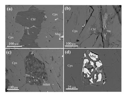
**Figure 6.** Chlorite in the samples of clinopyroxene I. (**a**) Interstitial chlorite (Chl) in clinopyroxene (Cpx). Chlorite also contains titanite (Ttn) and magnetite (Mag) in clinopyroxene; (**b**) veinlets of chlorite (Chl) with inclusions of titanite (Ttn) in clinopyroxene; (**c**) segregation of magnesio-ferrihornblende) (Mfhbl) in clinopyroxene. Amphibole is replaced by chlorite with titanite inclusions (Ttn); (**d**) magnetite crystal (Mag) replaced by chlorite (Chl) in clinopyroxene.
