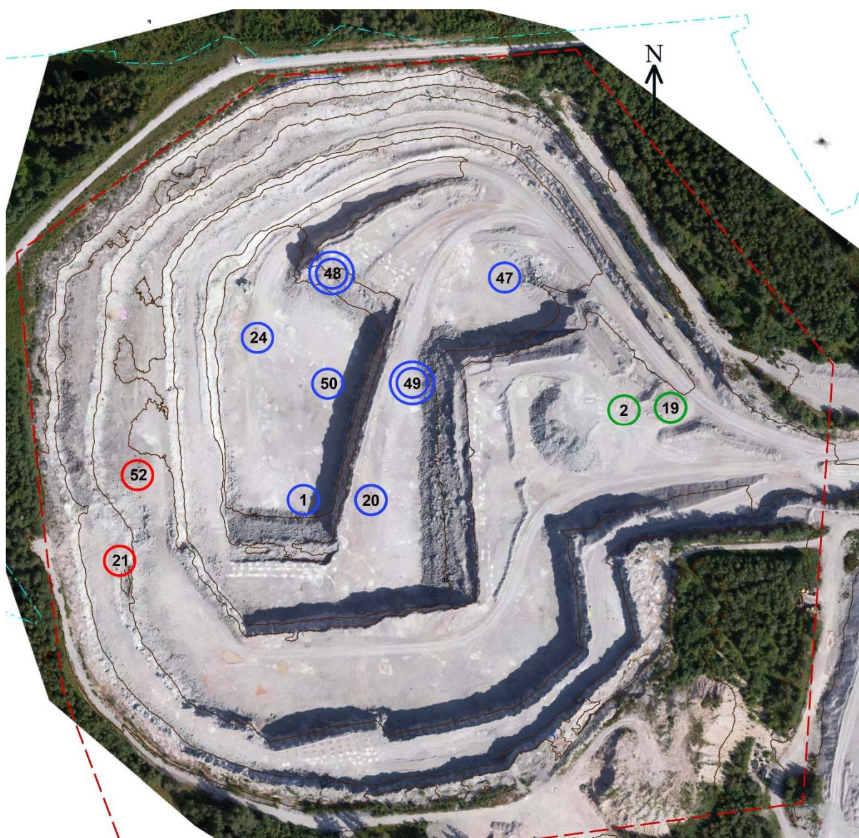
Figure 1. Aerial photograph of Jutjärn quarry. The boreholes are numbered, and the sampled boreholes are marked with a red, blue, or green circle. Two samples were taken from the double-blue-marked boreholes for further investigation of crack formation. For a more detailed regional geological map, visit: https://apps.sgu.se/kartvisare/kartvisare-berg-50-250-tusen.html?zoom=-1202129.5840071687,6016943.2639965275,2381877.5840071687,7752946.7360034725 (accessed on: 10 August 2022).
