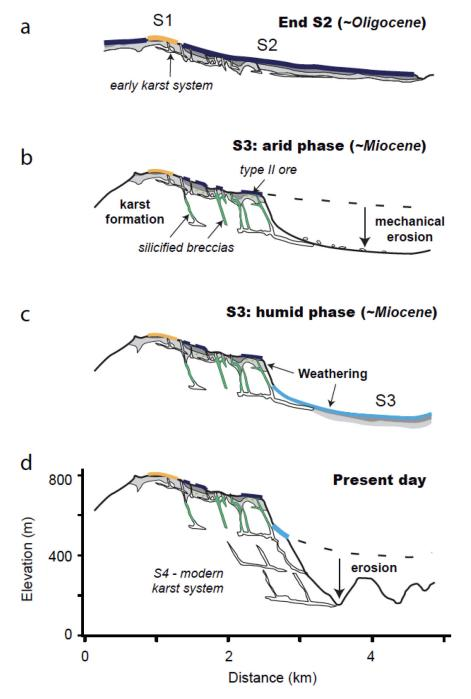
**Figure 11.** Conceptual model of the pseudo-karst development at Koniambo, with the paleosurface formation following the valley's deepening and progress in the erosion of the uplifted ophiolite.(a) Formation of the paleosurface S2 at the expense of S1, and initiation of the early karst system, (b) Deepening of the valley, and karst silicification during arid periods, (c) Formation of S3 related to humid periods, (d) Present day relief and karst.
