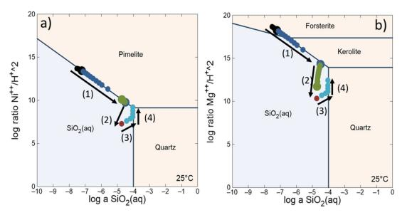
**Figure 15.** Chemical path of the mineralogical evolution in fractures in activity diagrams. (a) the  $Ni^{2+}/(H^+)^2 - SiO_2$  and (b)  $Mg^{2+}/(H^+)^2 - SiO_2$ . In colours, the predominant species in the system: Black: Olivine; Blue: Mg-Kerolite; Green: Pimelite; Red: Goethite; Light Blue: Quartz. (1) Progressive silicate dissolution. (2) Goethite dissolution in the overlaying laterite. (3) Evaporation up to quartz saturation. (4) Evaporation up to pimelite saturation.
