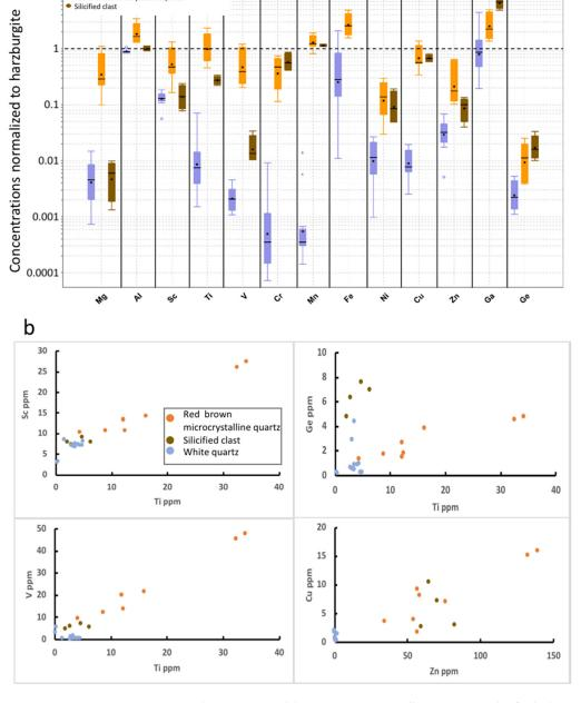
**Figure 8.** Trace elements in red-brown microcrystalline quartz, silicified clast and white quartz cement. (a) Normalised concentrations to harzburgite concentrations. (b) Binary plots, Sc-Ti, Ge-Ti, V-Ti and Cu-Zn for the three types of quartz.
