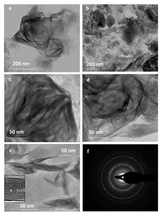
**Figure 7.** (a) TEM images of the Ni-silicate (pimelite). (b) Pimelite and euhedral quartz. (c,d) Flexuous assemblage of small size pimelite particles. (e) HRTEM image showing that the number of talc-like layers is generally low, about 5 to 15 in each particle, with no interstratification with other minerals. Indicative layer spacing is provided. (f) Diffraction pattern of one pimelite particle, with talc-like spacing.
