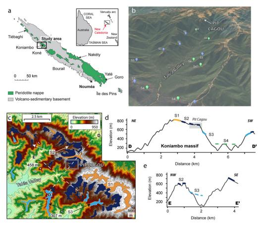
**Figure 1.** (a) Location of New Caledonia and Koniambo. (b) Aerial view with the indication of paleosurfaces (S1 to S4). (c) Location of the study site (open pit Cagou from KNS mining company) in the Koniambo massif. (d,e) Cross sections are in (c) (D-D' and E-E'), with the indication of S1, S2, S3 paleosurface (in yellow, dark blue and light blue respectively) and the potential location of S4 (green dashed line).
