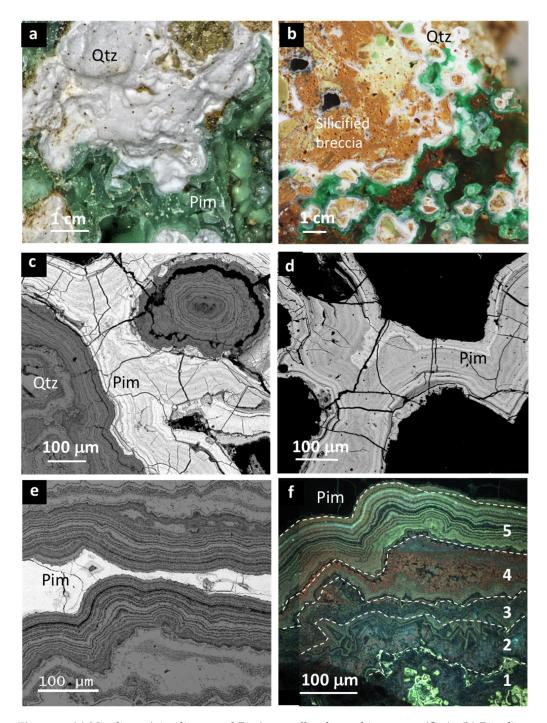
**Figure 4.** (a) Ni-silicate (pimelite, noted Pim) crystallised on white quartz (Qtz). (b) Pimelite on white quartz cementing silicified clasts. (c) BSE image showing the rims of quartz flowed by pimelite. (d) Detail of the chemical zoning in the pimelite colloform textures. (e) White quartz observed by BSE, showing a decreasing size of crystals; (f) Cathodoluminescence image showing white quartz rims from 1 (earliest rim) to 5 (colloform quartz).
