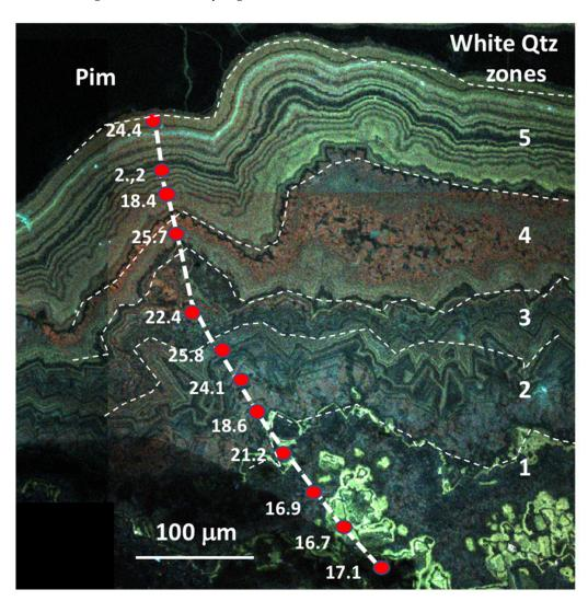
**Figure 9.**  $\delta^{18}O$  (‰) values along a profile crosscutting white quartz from silicified breccia to the centre of the cavity (Zones 1 to 5). The colloform pimelite appears in black in the central vug.  $\delta^{18}O$  values are reported on the cathodoluminescence image.
