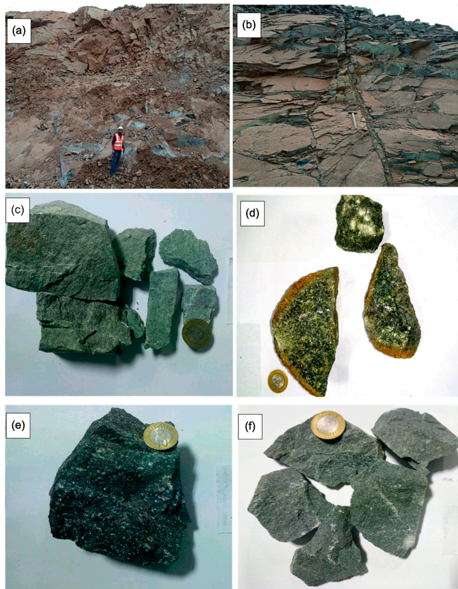
Figure 2. (a,b) Field photographs of ultramafic rocks exposed in Sukinda chromite mines. (c,d) Ultramafic hand specimens collected from the Kaliapani area. (e,f) Ultramafic hand specimens collected from the Katpal area.
