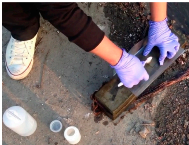
Figure 1. Removal of chlorophyll-a from the cement mortar specimen immersed in sea.
