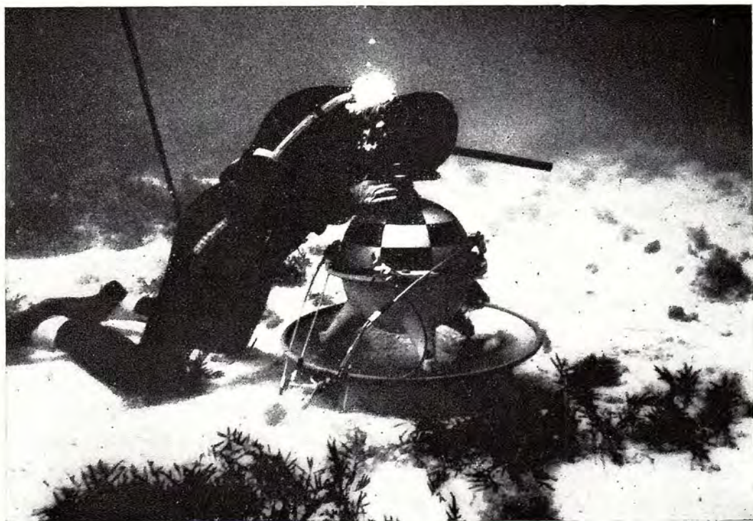
A geophysicist metering sea-floor gravity in Spencer Gulf, South Australia, in a search for dense bodies likely to relate to ore bodies. [Photo: Mrs J. Watson.]
