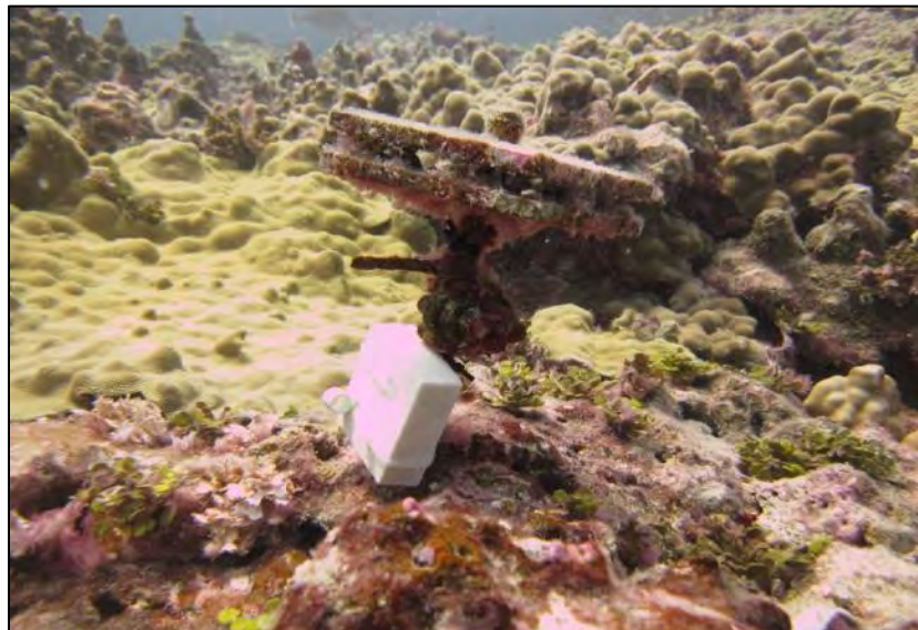
Figure A-20 Bioerosion monitoring block with CAU unit
