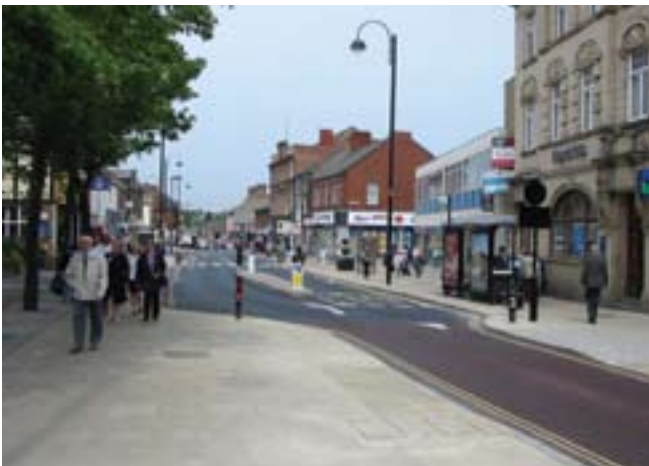
Classic precast concrete paving flags can play an important part of urban design, here with tactile paving at crossings and wider footways to improve the pedestrian environment
