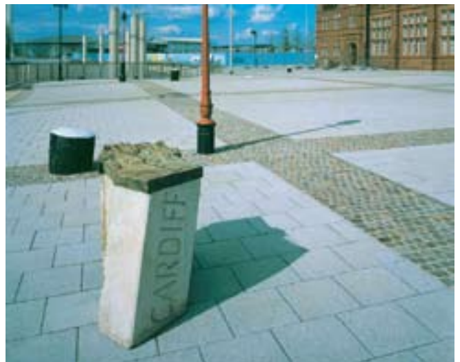
Interpave manufacturers work in partnership with local authorities to develop specific products and finishes to give local identity – in this case, a special paving flag for the Cardiff Bay area redevelopment
