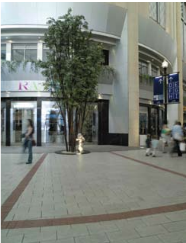
Precast concrete paving can also be enhanced with a high quality honed decorative finish, in this case used internally
