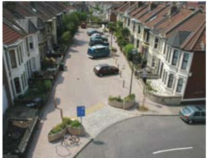
Differentiation of paving surfaces with other features is used to form gateways to Home Zones, as in this Bristol example
