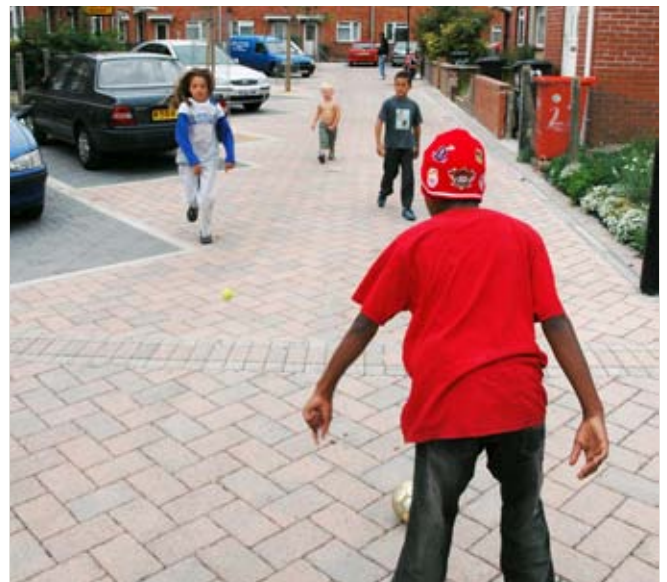
Concrete block permeable paving, combined with conventional block paving, is used throughout this major regeneration project in Craigmillar, Edinburgh.
