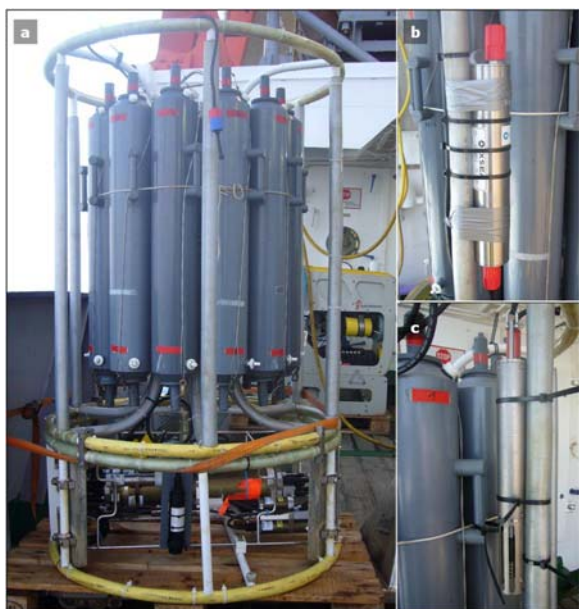
Fig. 4.1 A CTD onboard RV Poseidon . The CTD frame was additionally equipped with B a GAPS transponder to calibrate the positioning of the ROV, and C a sound velocity sensor to get sound velocity profiles to calibrate the MBES.
