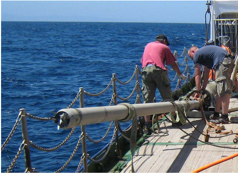
Fig. 3.7 Bent core tube, a so-called 'banana'.
