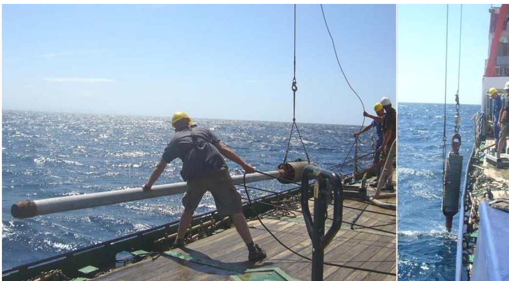
Fig. 4.4 Deployment of a gravity corer with a 6 m long pipe on board RV Poseidon .
