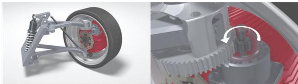
Figure 2.3: The wheel robot with in-wheel actuators and suspension (left); The wheel carrier mounted steering mechanism (right)
