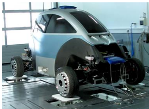
App. Figure B.6: ROMO on a four-post test rig
