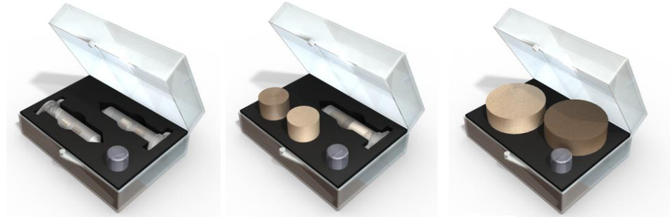
Figure 2. Bruker-MicroCT BMD calibration rod pairs are provided in a range of diameters (2-4mm, 8-16mm, 32mm) to match the size of the scanned bone.
