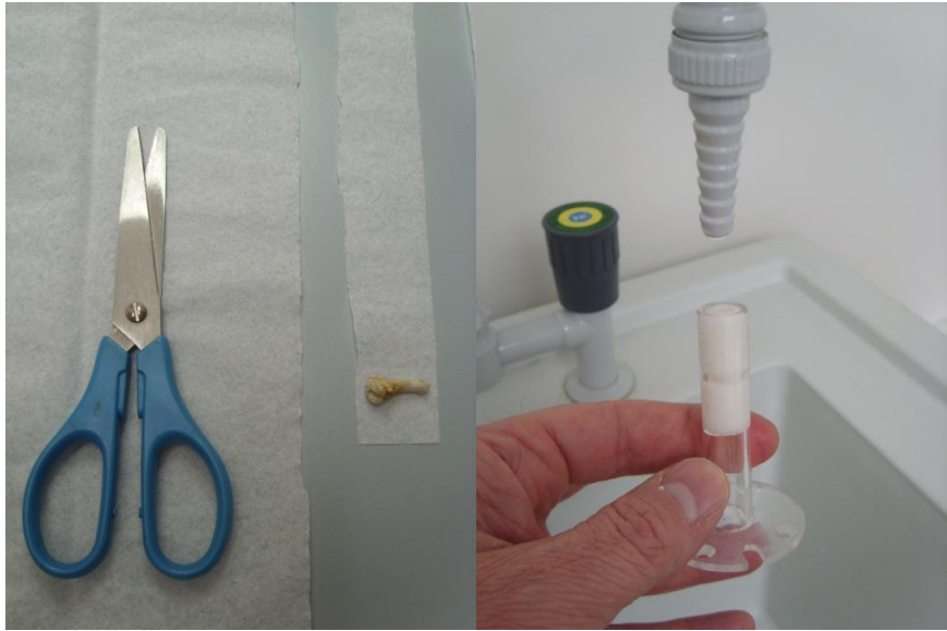
Figure 6. To maintain hydration of bones during a scan, one option is to wrap the bone in paper tissue for placement in a suitable plastic tube holder, then moisten the paper tissue with tap water or alternatively saline. This will effectively keep the bone moist during a scan.
