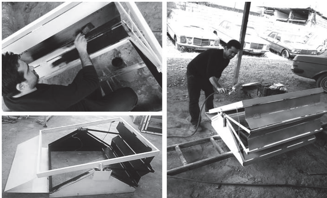
FIGURE 12. The inner sides of the system was covered with black for absorbing sun radiation.
