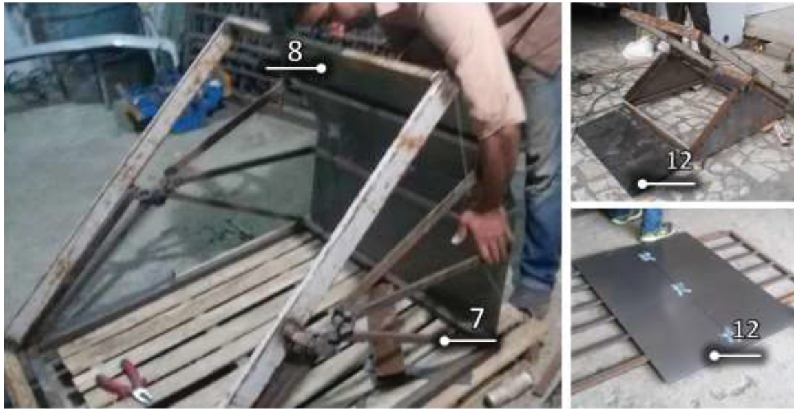
FIGURE 11. The folding panel placed on top of the system and its details.
