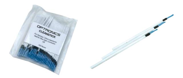
Micro fibre sticks are the ideal consumable for cleaning 1.25mm bulkheads after installation. They can be used to clean the end faces of installed connectors, from inside the enclosure. Cleaning is achieved by inserting the micro fibre tip inside the adapter's aperture and twisting once.
