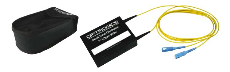
OTDRs require launch and receive test cables to measure the end-to-end loss of optical fibre links. A launch cable, which connects to the OTDR to the link under test, reveals the insertion loss and reflectance of the near-end connection. A receive cable, which is connected to the far-end of the link, reveals the insertion loss and reflectance of the far-end connection.
