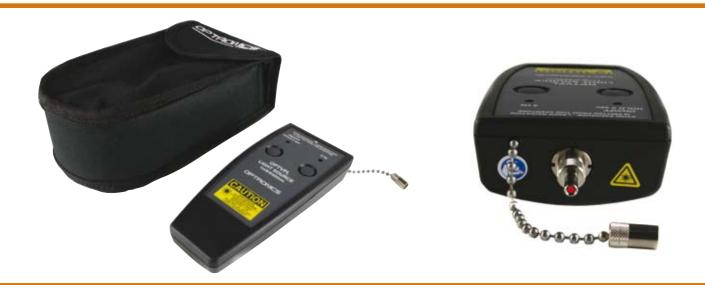
The OPTVFL is a compact but powerful visual fault locator, designed to troubleshoot faults on fibre optic cables. Light generated by this unit will escape from sharp bends and breaks in jacketed or bare fibres, as well as poorly mated connectors. It can also identify faults in fibre optic cables, distribution frames, patch panels, and splice trays.
