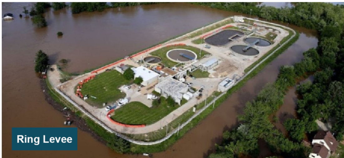
Figure 2-8: Typical Ring Levee
