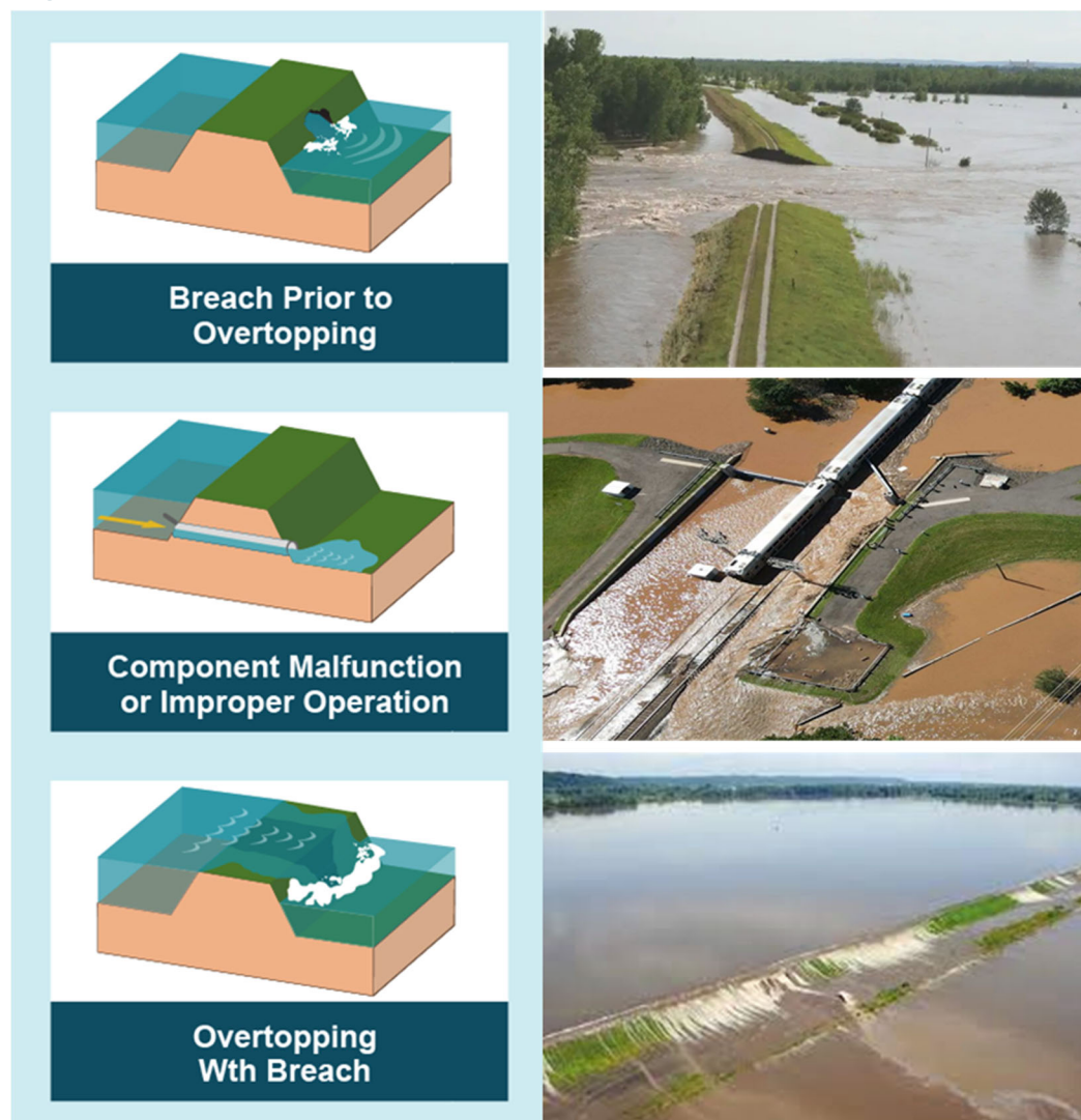
Figure 2-46: Levee Breach Scenarios
