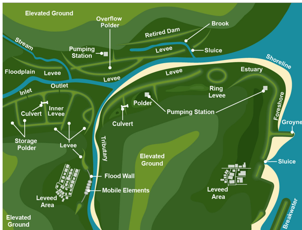
Figure 2-5: Typical River Levee
