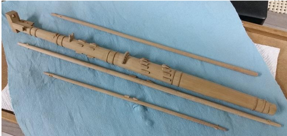
Figure 3 - (from top to bottom) Jib Boom, Bowsprit, Sprintsail Yard, and Sprintsail Topsail Yard
