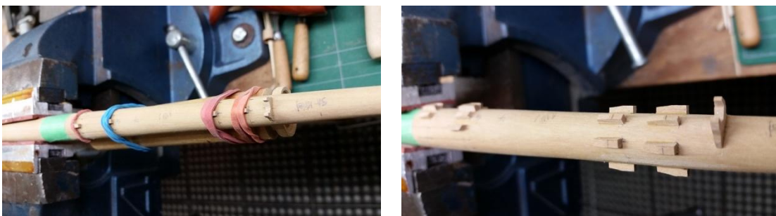
Figures 13 & 14 - Installing and clamping the Thumb Stop Cleats
