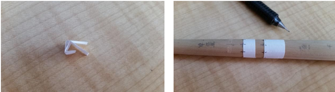
Figures 11 & 12 - Templates to locate the Thumb Stop Cleats
