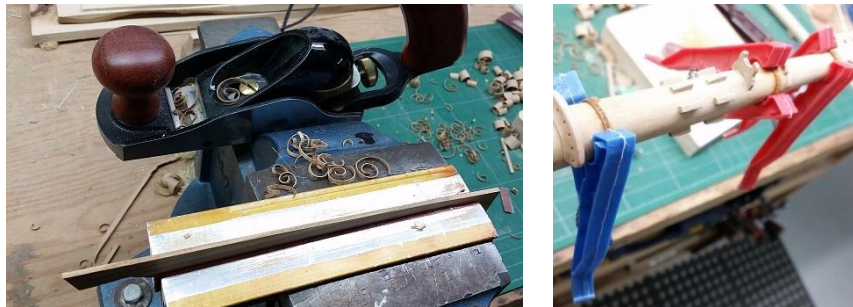
Figures 16 & 17 - Planing and installing/clamping Woolding Hoops
