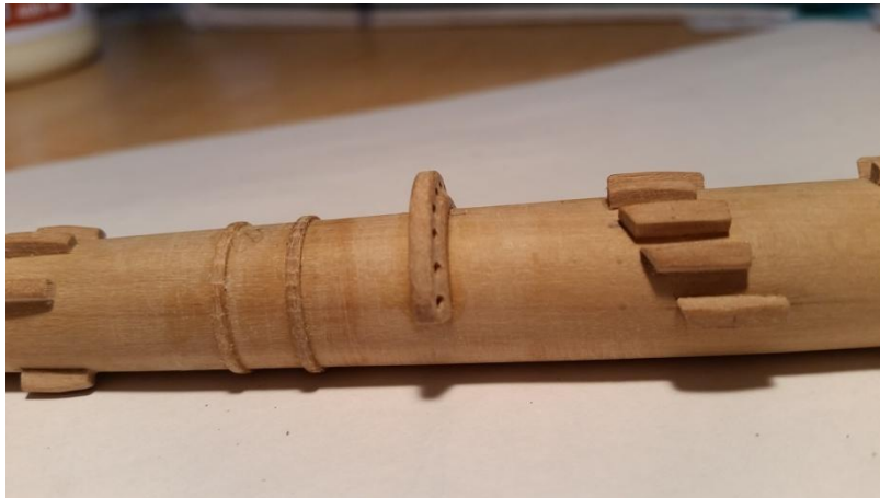
Figure 25 - New Fairlead Saddle Installed
