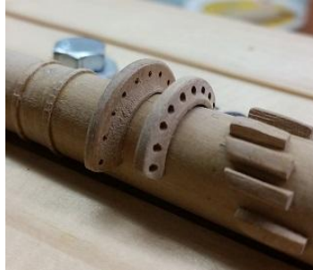
Figure 19 – First (left) and replacement (right) Fairlead Saddles
