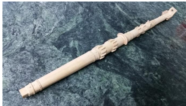
Figure 18 - Woolding Hoops Installed
