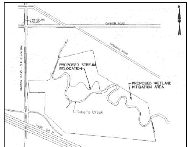
Figure 1: The Tinker's Creek channel relocation necessary to make way for construction of Creekside Plaza, Twinsburg, Ohio.
