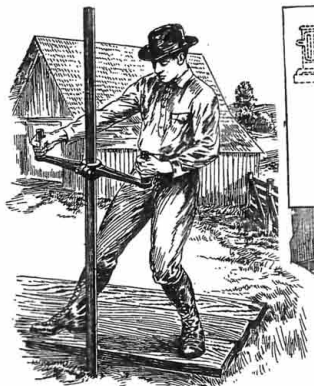
Adjustable Handle Facilitates Work of Boring Shallow Wells by Hand
