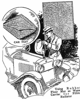
Emergency Filler for Radiator
