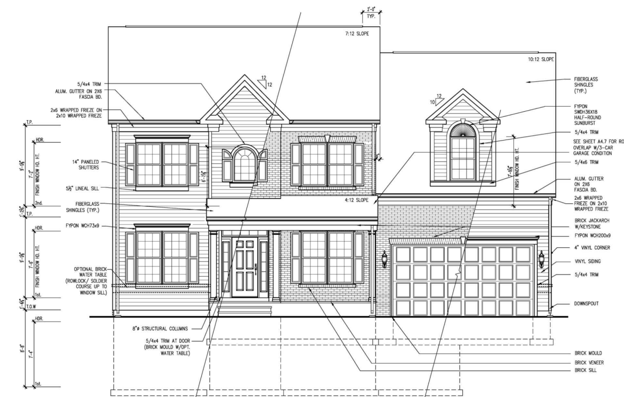
FRONT ELEVATION 1 W/OPT. EXTENDED PORCH NOTE: OPTIONAL EXTENDED FRONT PORCH TO BE STANDARD ON ELEVATION 1
