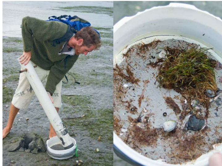
Figure 4.5. Left – core sampling, right – material retained after sieving.
