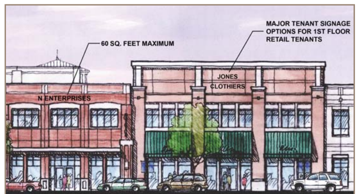
A MAXIMUM OF ONE SECOND FLOOR MAJOR TENANT SIGN IS PERMITTED PER SECOND FLOOR TENANT. SIGNAGE MAY BE MOUNTED TO THE PARAPET, BUT MAY NOT PROJECT ABOVE THE PARAPET CAP.
