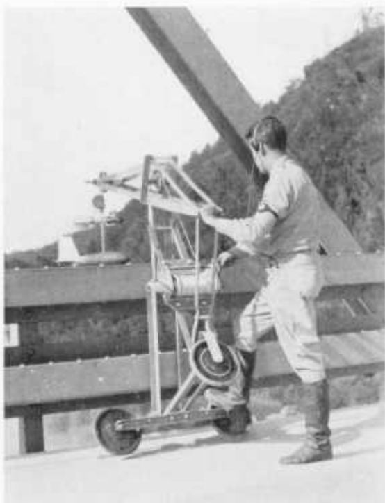
PLATE 2, FIG. 2. Equipment Used in Making Discharge Measurements from Bridge.
