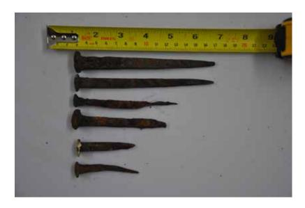
FIGURE 5 Fort Alice's forged steel nails retrieved during the conservation, 2013. (Photograph reproduced with the permission of Arkitek JFN)
