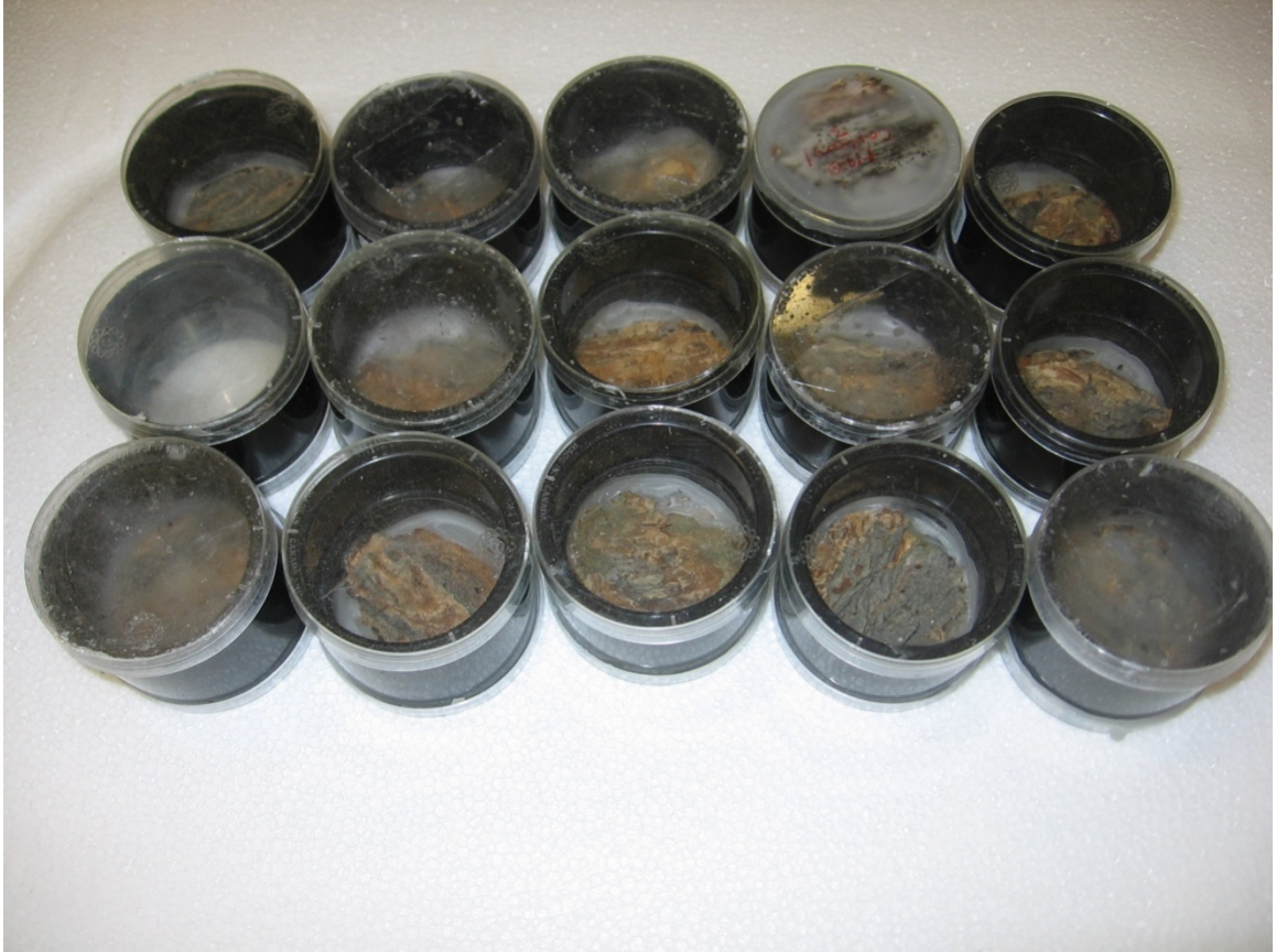
Figure 24. Modified PVC pipes with bark disk floors used as bioassay chambers. Photo credit: Sunday Oghiakhe.
