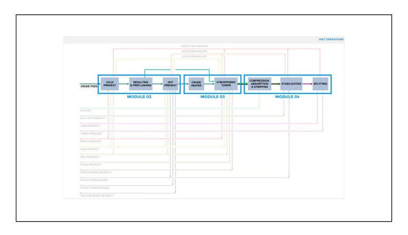
Here's the overall block flow diagram for the ADU that we introduced in module 1. You'll recall that the ADU has 8 distinct unit operations - we've divided these into topics which will be covered in ADU Modules 2, 3 & 4.
