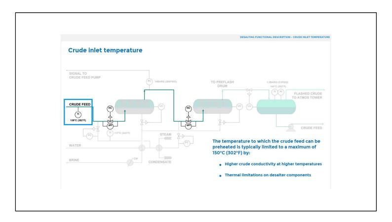
Temperature plays an important role in desalting - maximizing the crude preheat temperature minimizes the crude viscosity - this accelerates the coalescence and settling of water droplets, which improves desalting efficiency.
