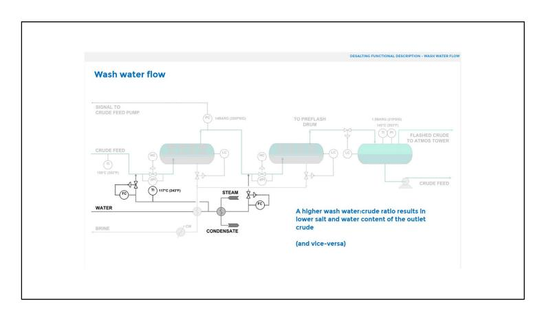
The flow of wash water to each desalter is controlled in proportion to the crude feed rate. A higher wash water:crude ratio results in lower salt and water content of the outlet crude (and vice versa).
