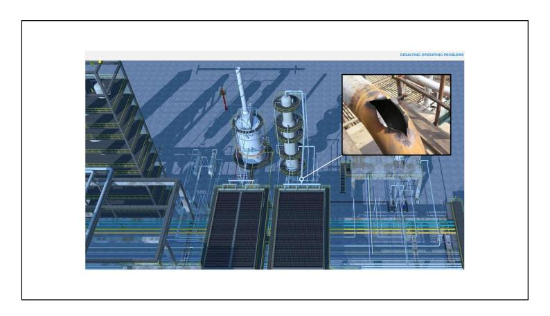
Taken from our NHTU archives, here's an example of the extent of hydrogen chloride and ammonium chloride corrosive attack.
