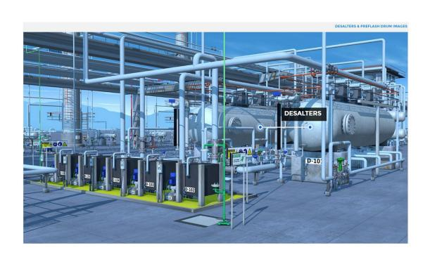
The 2-Stage Desalters are large horizontal vessels (like the ones pictured here), usually located next to the preheat exchangers. The Preflash Drum is similarly sized.
