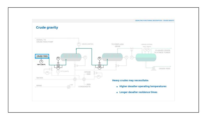
Heavy crudes (which are characterized by increases in specific gravity, viscosity and conductivity) may necessitate:
