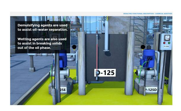
Many refineries use chemical additives in the desalting process.
