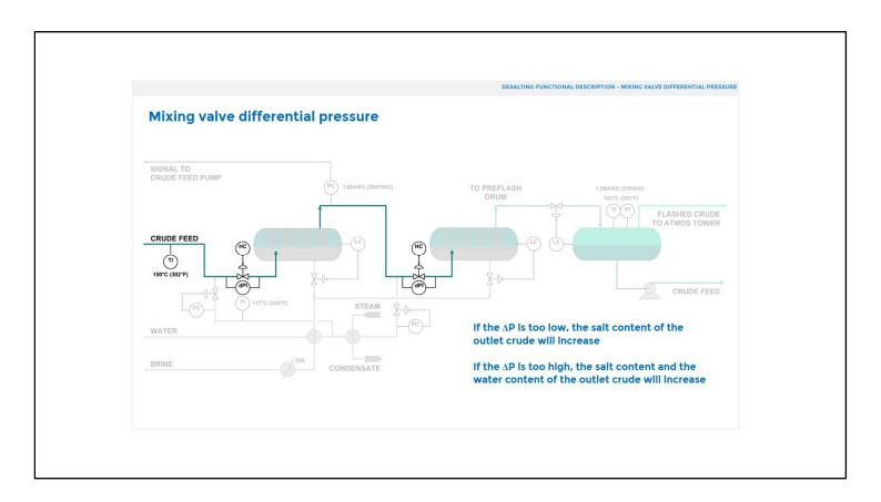
The  $\Delta P$  across the mixing valve ensures that the wash water is fully distributed throughout the crude:
