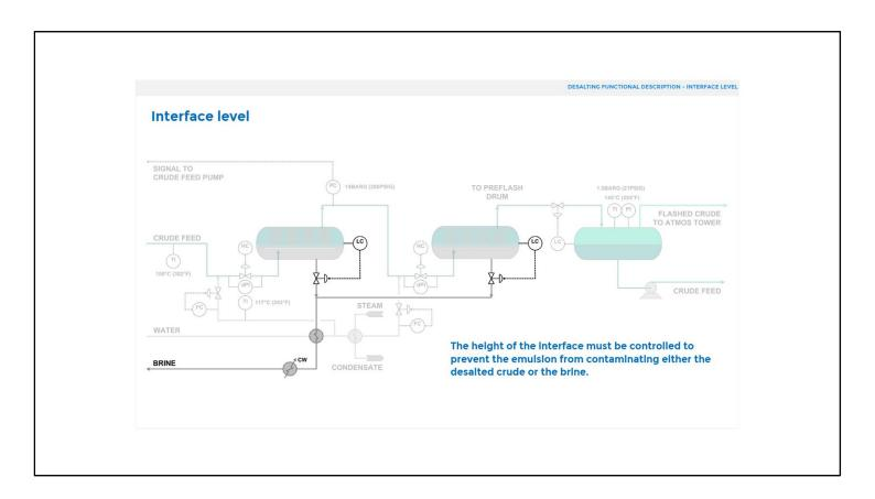
The Desalter interface level is an important variable - the desalters are operated full, with oil at the top and water at the bottom, separated by an emulsified oil-water interface.
