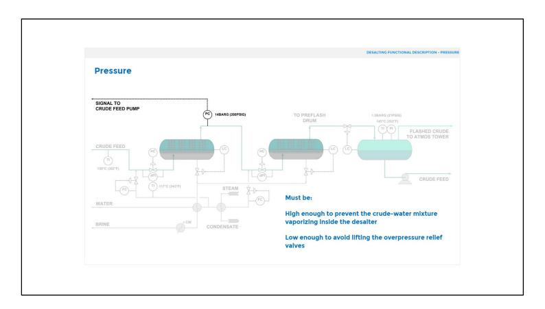
Pressure does not affect desalting efficiency, except that it must be:
