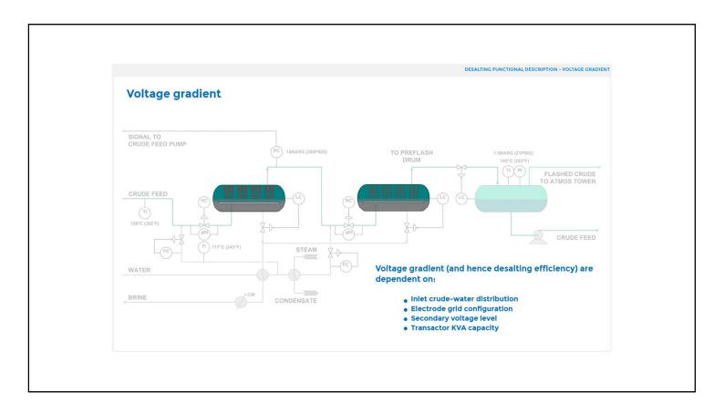
The voltage gradient between the electrode grids inside the desalter provides the driving force for water droplet coalescence. Voltage gradient (and hence desalting efficiency) are dependent on:
